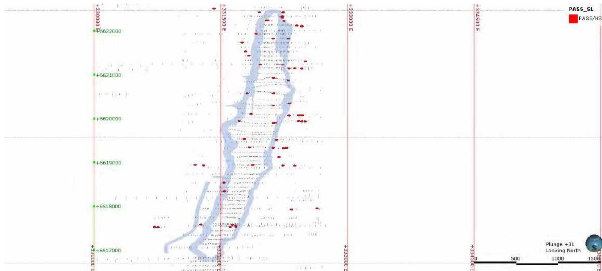
Figure A2 Drillholes logged with a combination of PASS (based on dark soil colour) and high clay fines content (HSL)
