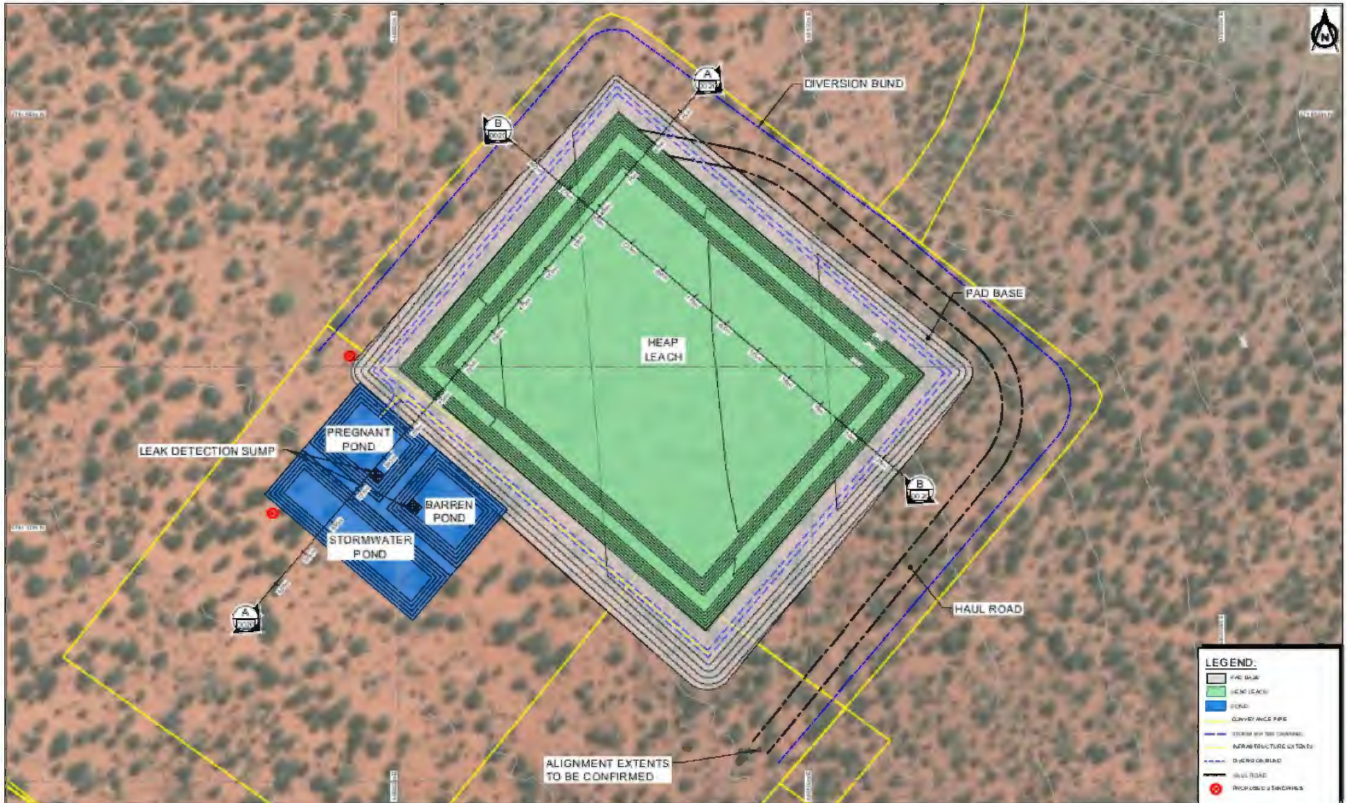
Figure 7: Heap Leach Pad and Pond Design (Courtesy – Tailex)
