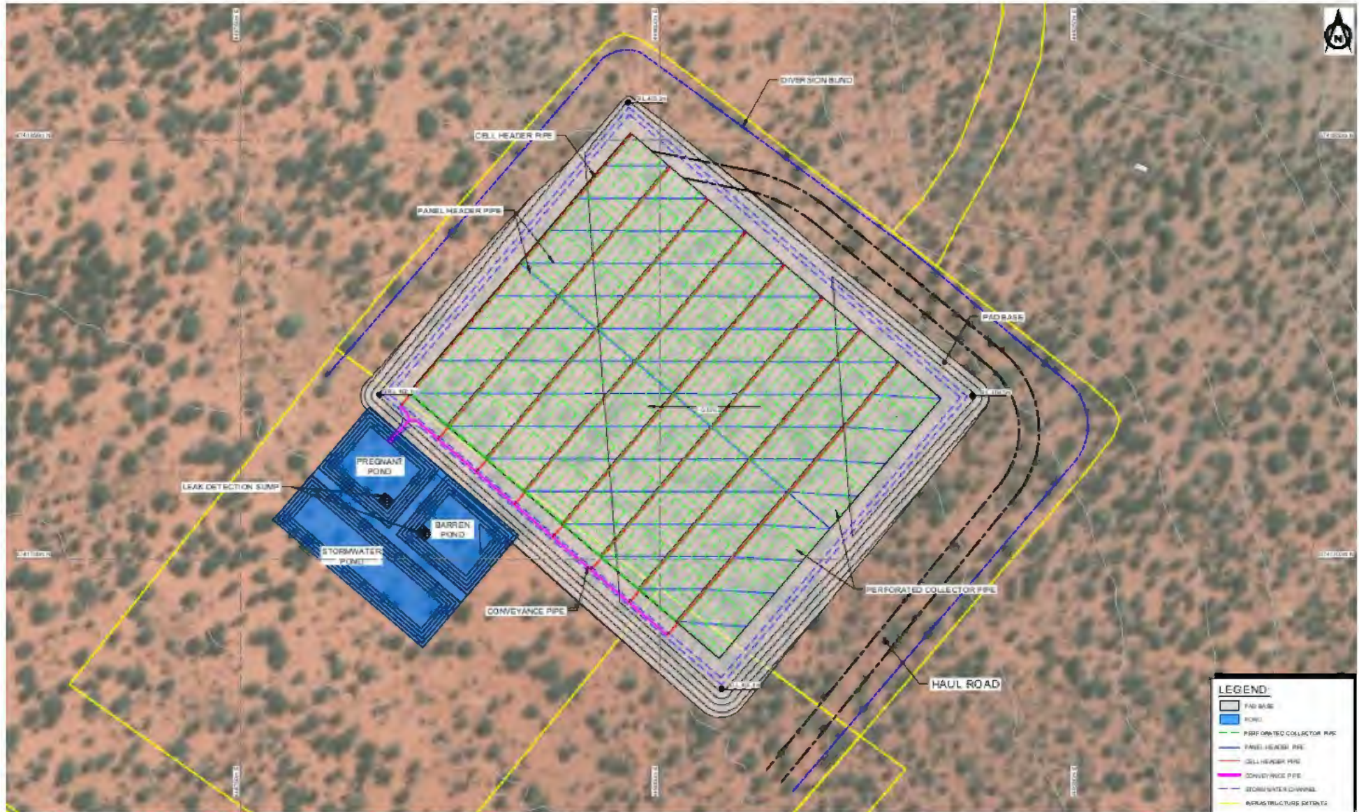
Figure 8: Heap Leach Pad Drainage Design (Courtesy – Taillex)
