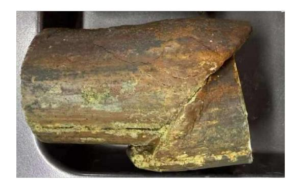
Failure Mode: Intact Shear @ 37.3°
