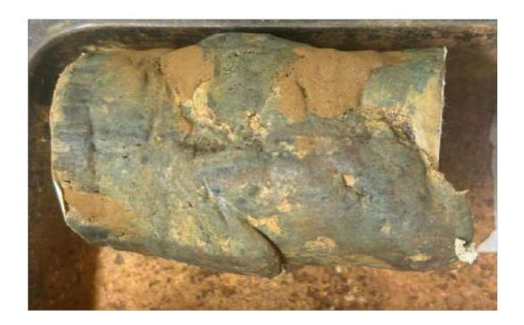
Failure Mode: Intact Shear @ 29°
