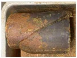
Failure Mode: Intact Shear 36.3 °
