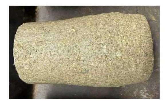
Failure Mode: Bulging Failure
