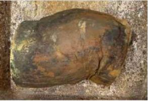
Failure Mode: Intact Shear 27 °
