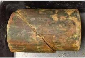
Failure Mode: Intact Shear 46.6 °
