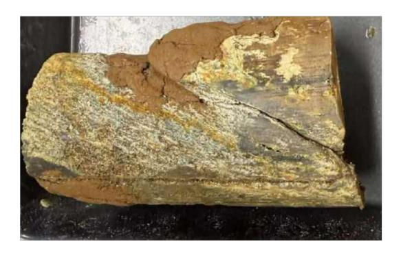
Failure Mode: Intact Shear @ 26.5°
