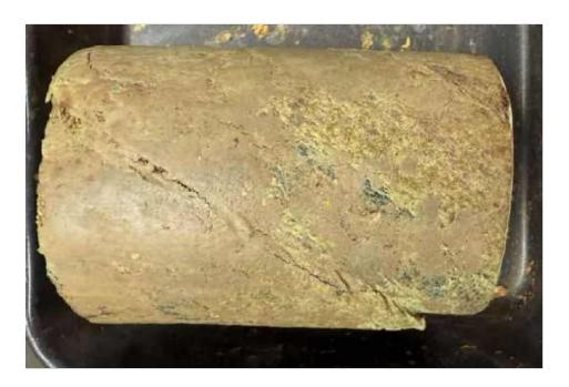
Failure Mode: Intact Shear 32.6 °
