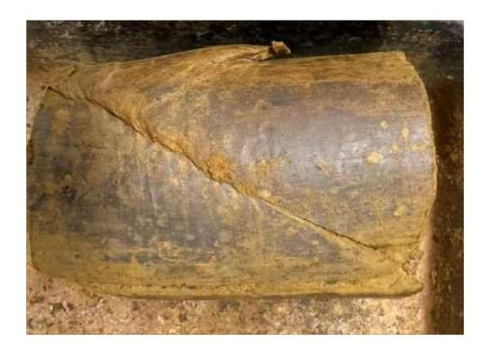
Failure Mode: Intact Shear @ 36.6°
