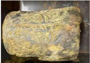
Failure Mode: Intact Shear 32.5 °
