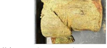
Failure Mode: Intact Shear 42.5 °
