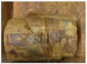
Failure Mode: Intact Shear 35.6 °
