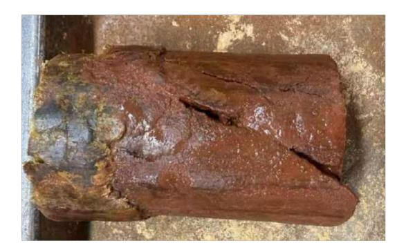
Failure Mode: Intact Shear @ 35.8°
