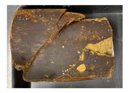
Failure Mode: Intact Shear @ 37.6°
