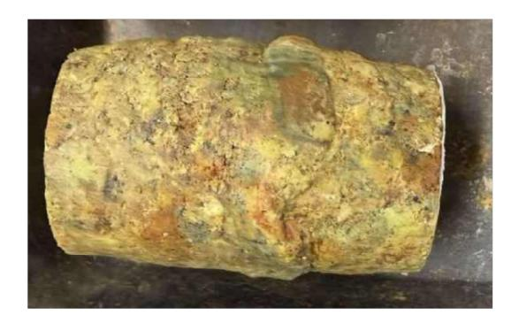
Failure Mode: Intact Shear @ 24.7°
