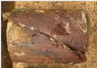
Failure Mode: Intact Shear 32.2 °
