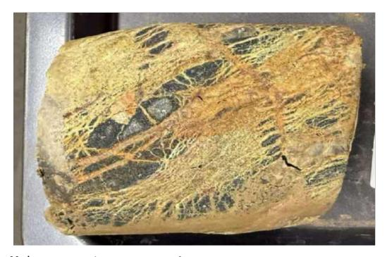
Failure Mode: Intact Shear 38.6 °
