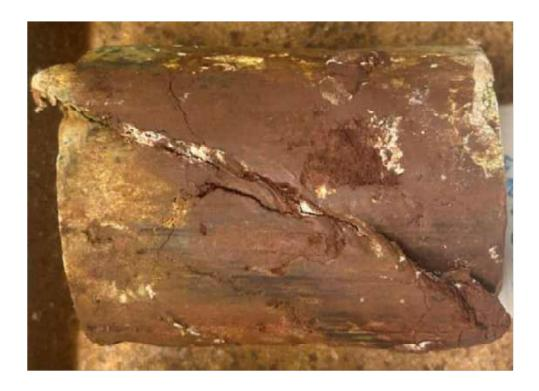
Failure Mode: Intact Shear @ 32.5°
