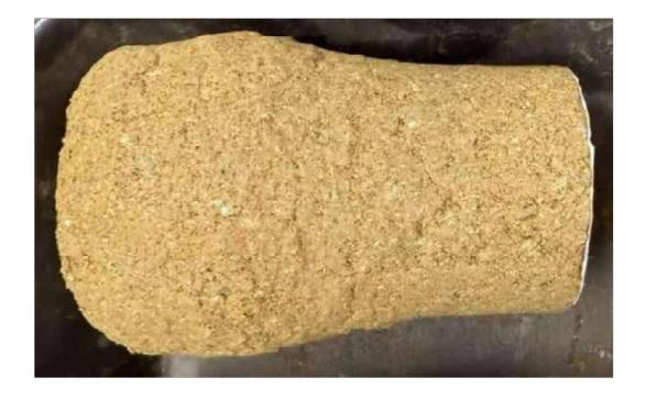
Failure Mode: Bulging Failure
