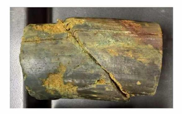
Failure Mode: Intact Shear @ 46.1°
