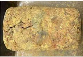
Failure Mode: Intact Shear 33.1 °
