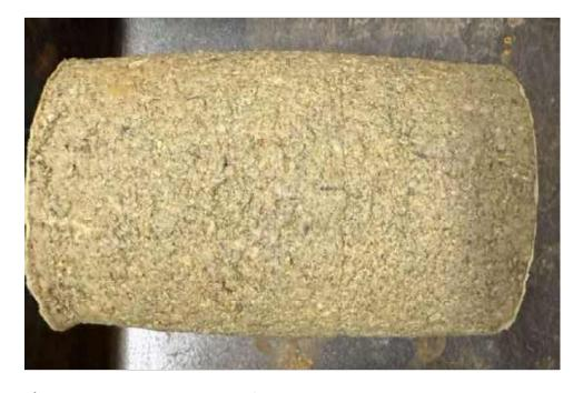
Failure Mode: Bulging N/A °
