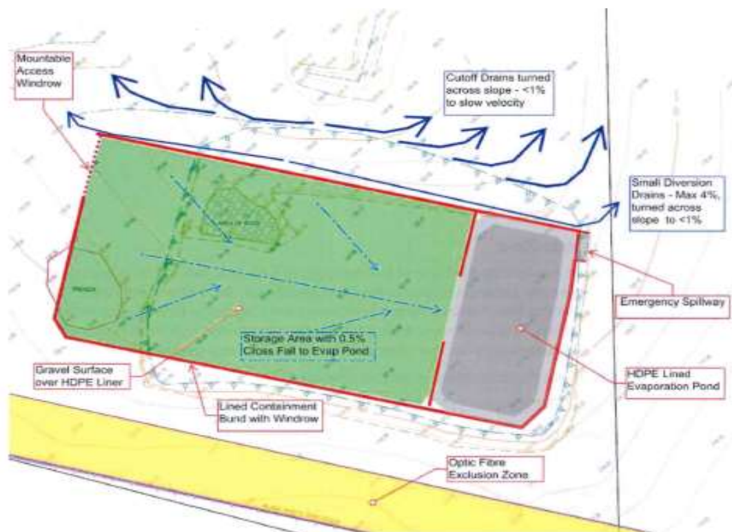
Figure 1: General arrangement of the bioremediation pad and evaporation pond
