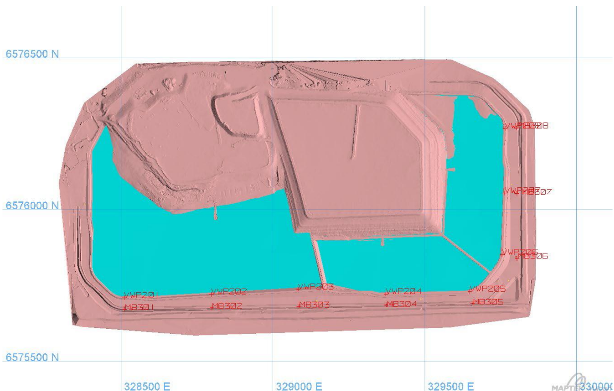
Figure 1: TSF3 cells (blue) with piezometers and monitoring bores
