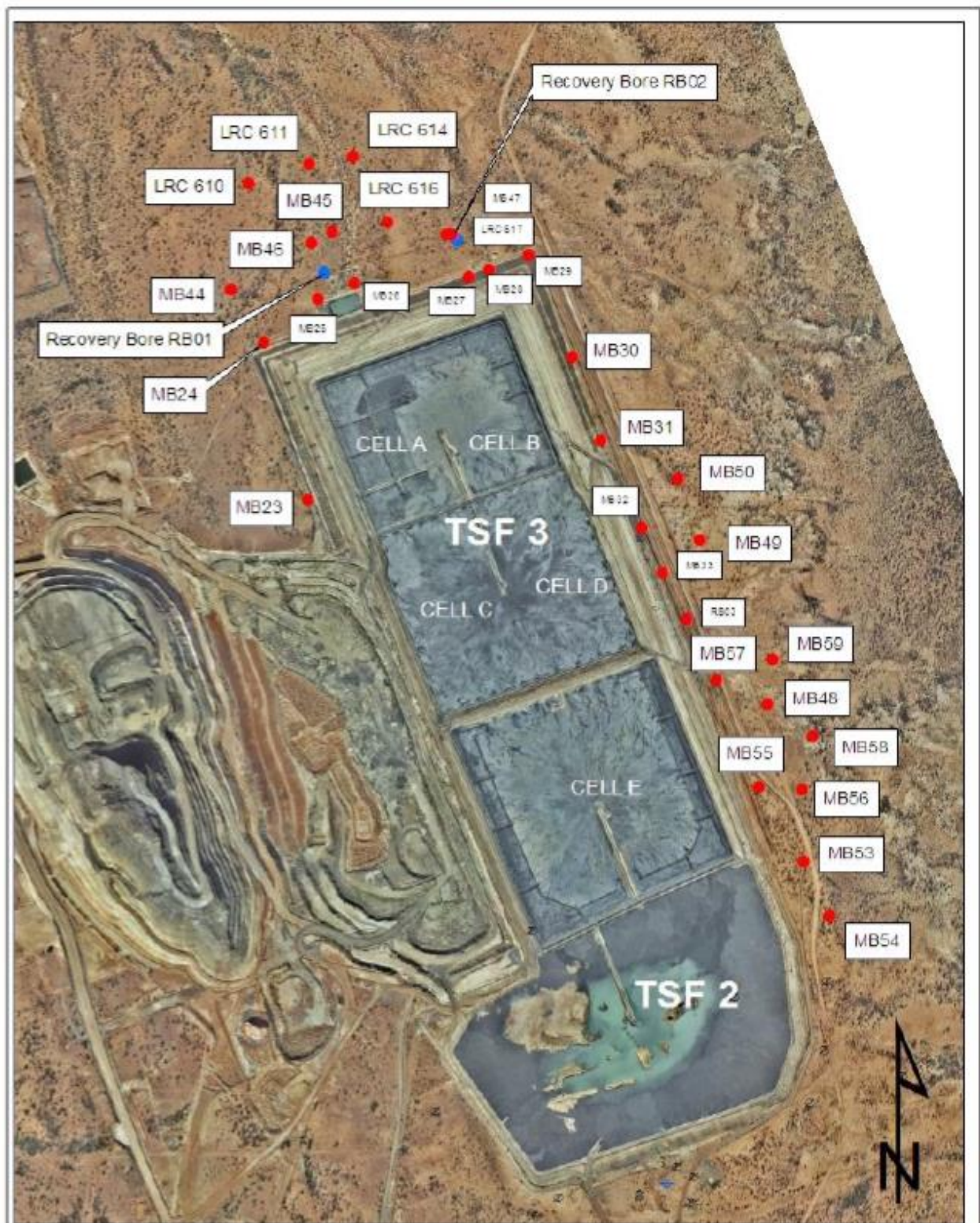
Figure 1: Nickel West Leinster Active TSFs (TSF2 and TSF3). Cell CD is shown with adjacent groundwater bores. Recovery bores RB01 and RB02 are shown to the north of TSF Cell AB. Recovery bore RB03 is also shown adjacent to Cell CD. This was installed in the 2001 but has not been operated due to low yields (Berry 2017).
