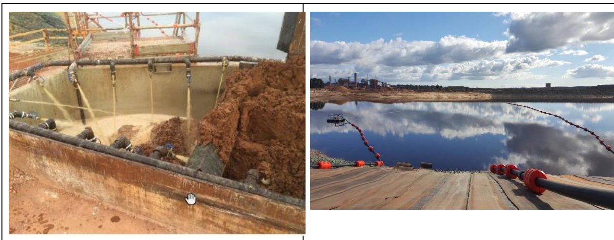
Figure 3: An example of the sprinkler operation within the hopper (photo left) and pontoon pump and floating slurry release line (photo right) that is proposed for SEP1
