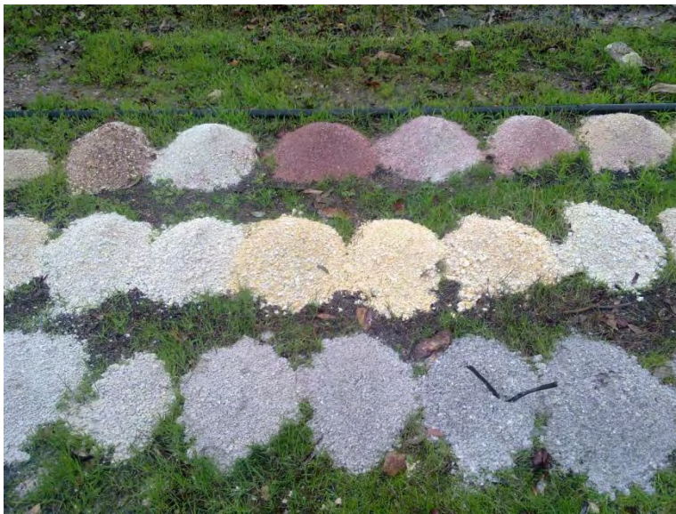
Photo plate 1 - Drill cuttings sampled at 1 m intervals. Water struck at 39 m depth.
