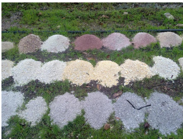
Photo plate 1 - Drill cuttings sampled at 1 m intervals. Water struck at 39 m depth.
