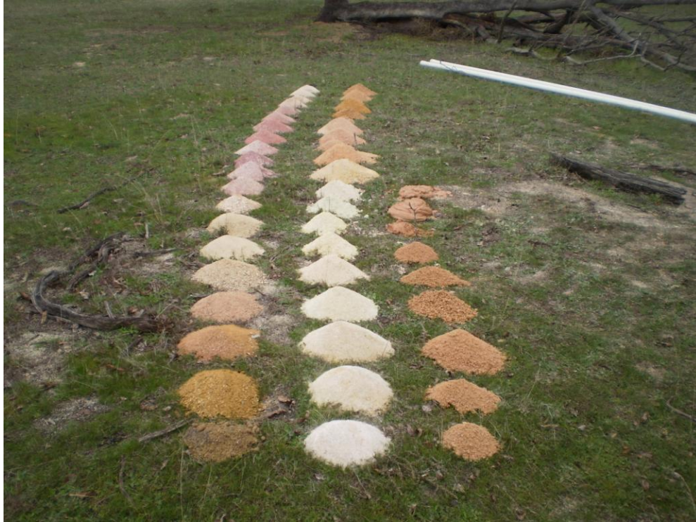
1 m interval sample record showing water intersected at the last 4 samples (46 m below the surface)
