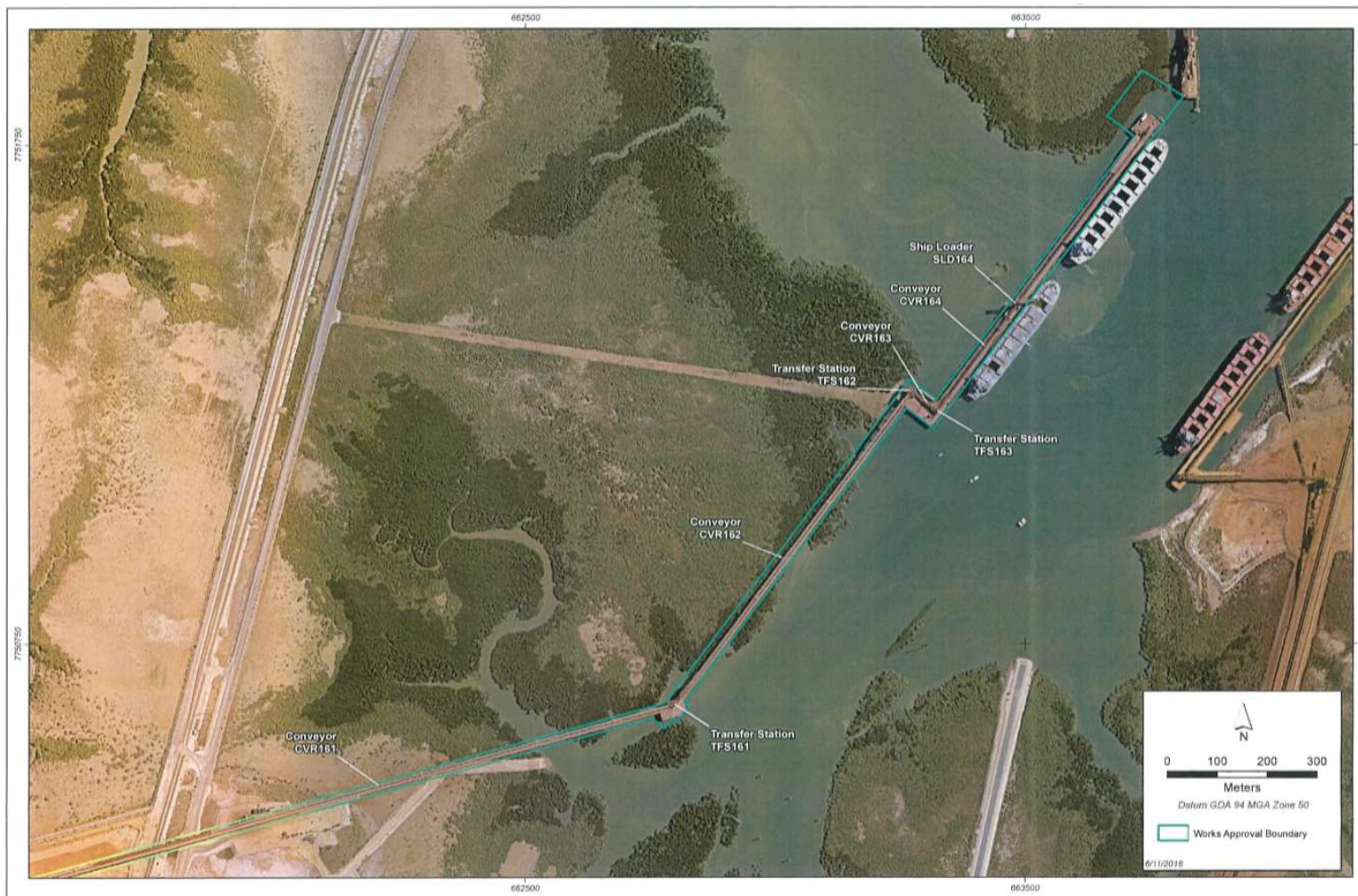
Figure 4: Overland conveyor and ship loading area layout
