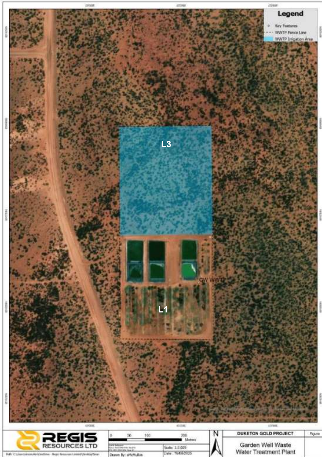
Figure 9: Map of the existing Garden Well WWTP irrigation field and ponds (L1 Emission point) and location of New Garden Well treatment ponds and irrigation field (blue area) (L3 Emission point)
