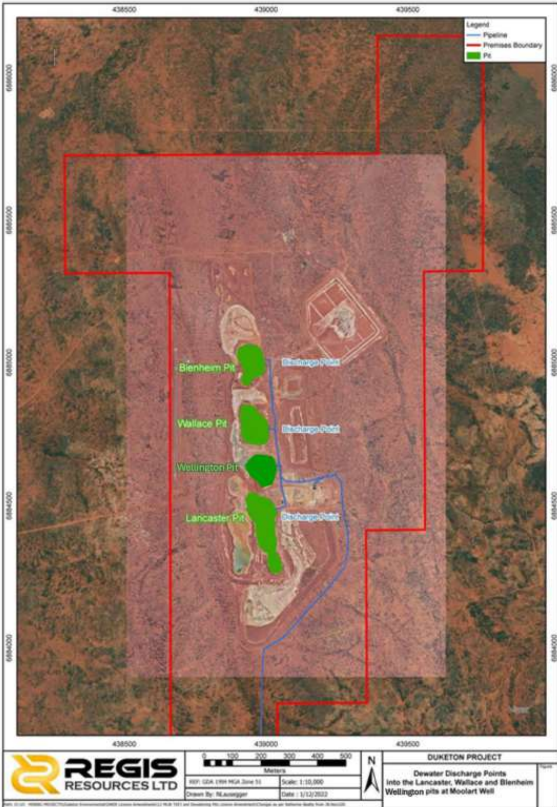
Figure 13: Map of dewater discharge points into the Lancaster, Wallace, Blenheim and Wellington pits at Moolart Well.
