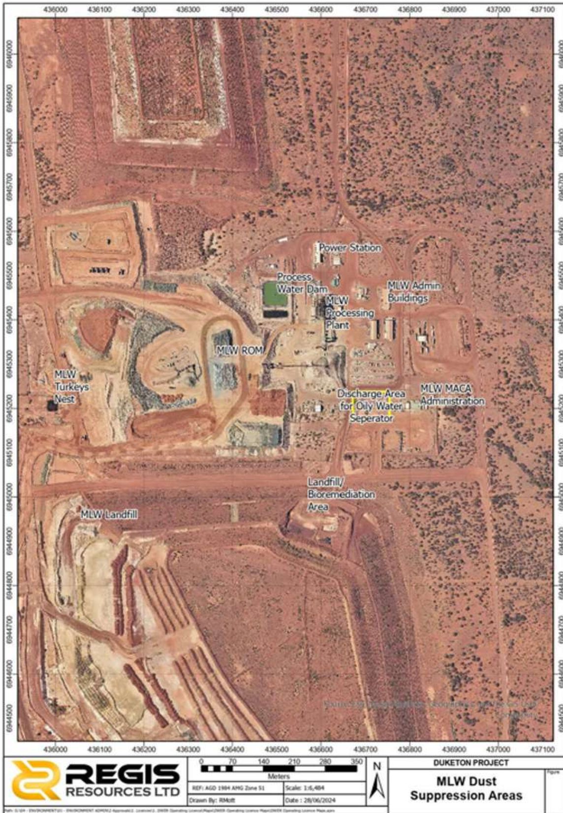
Figure 11: Map of approved area's where treated water from Moolart Well oily/water separator can be used for dust suppression as referenced in condition 16
