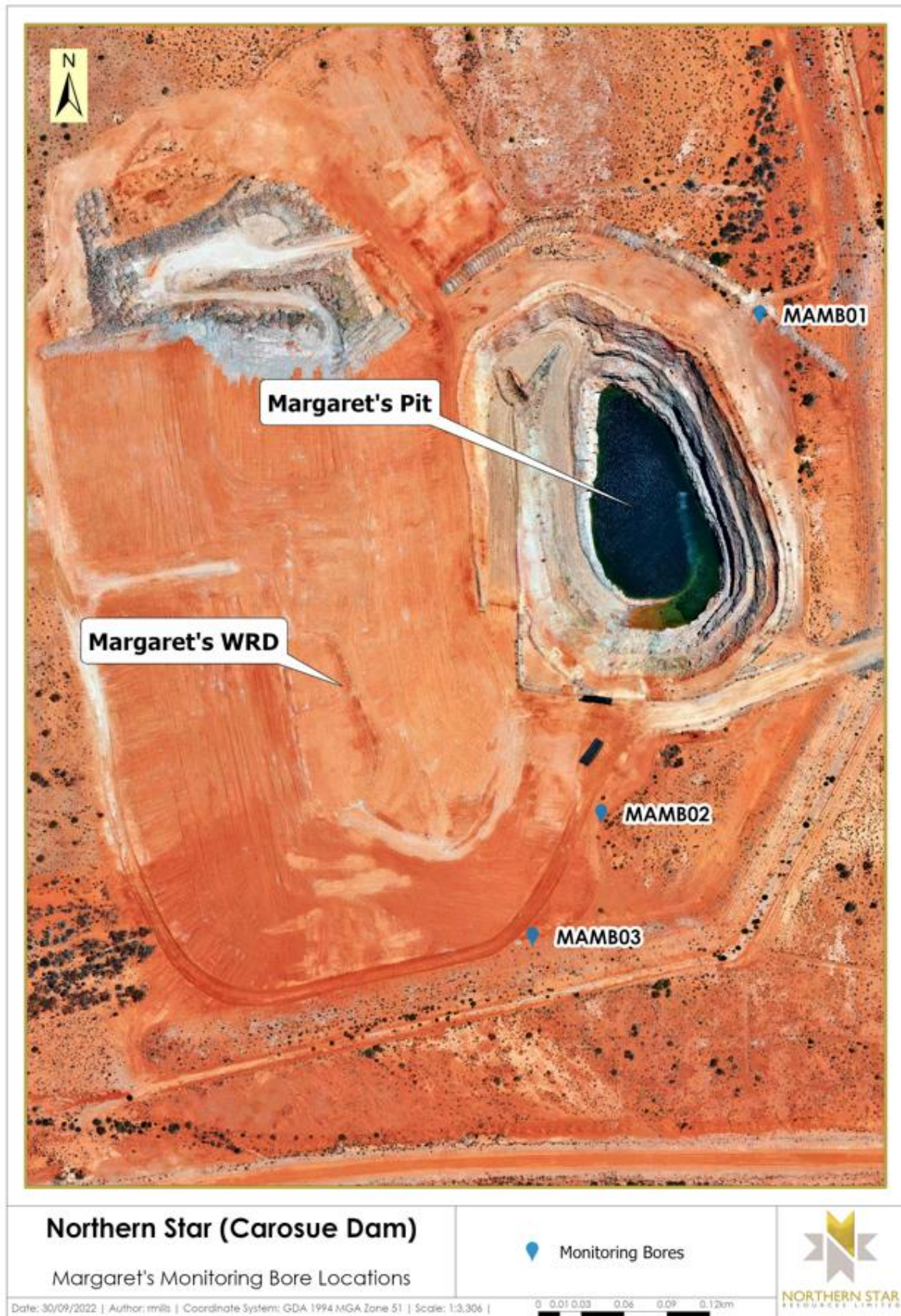
Figure 8. Margaret's pit monitoring bores
