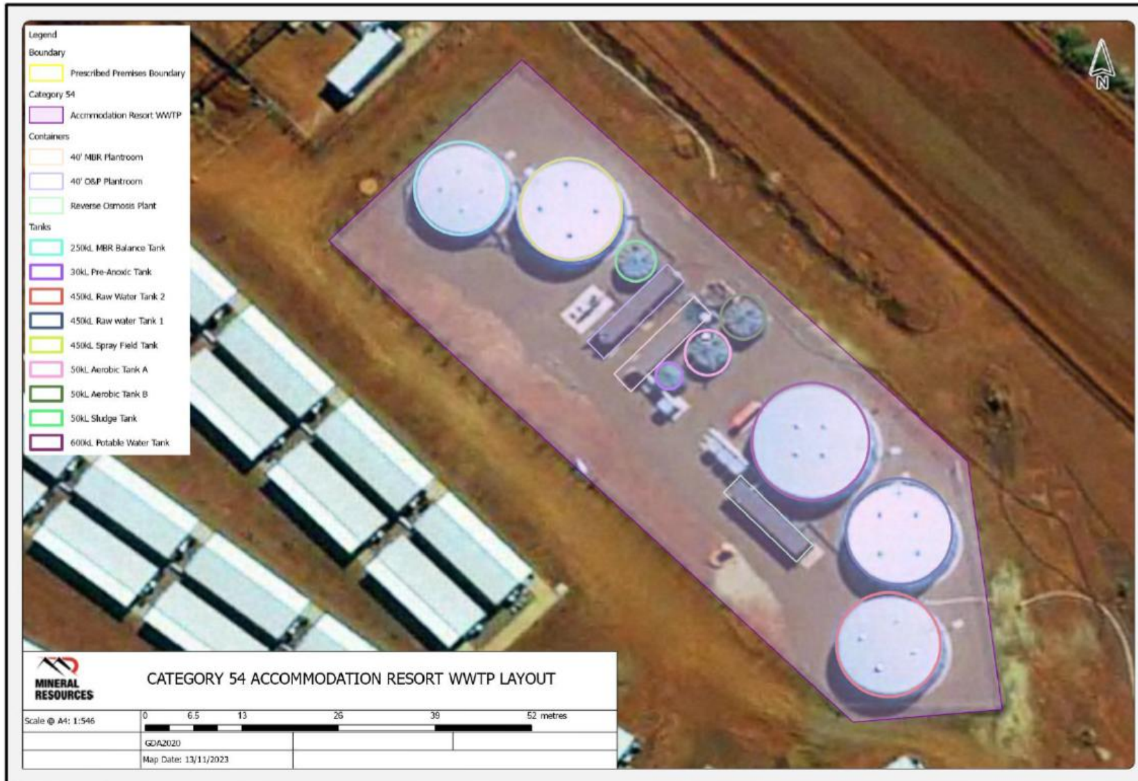
Figure 6: Layout of Accommodation Resort WWTP (200 m 3 /day)
