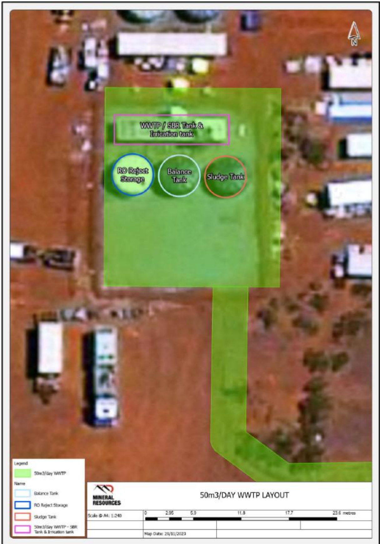
Figure 7: Layout of Construction Camp WWTP (50 m³/day)
