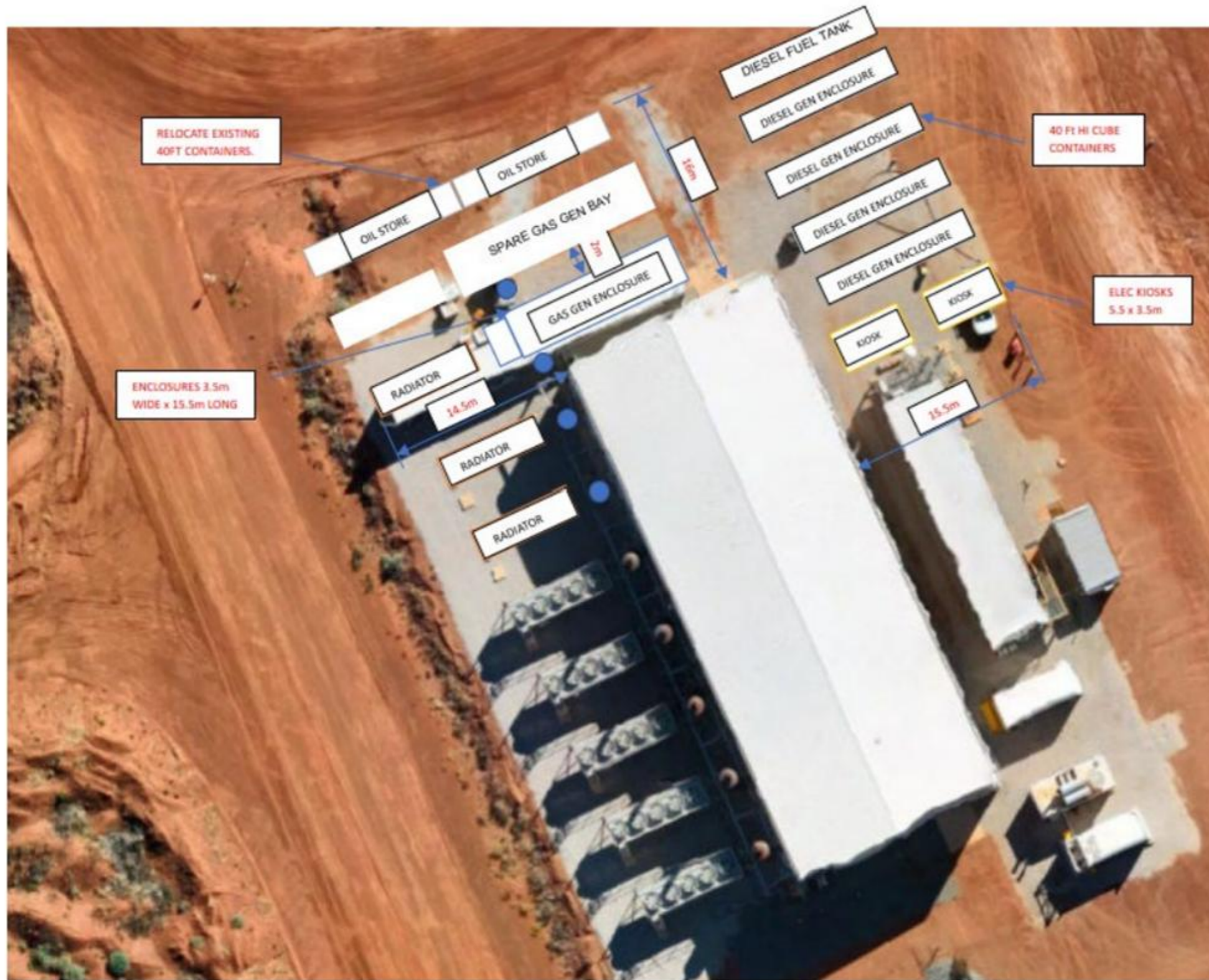
Figure 3: Power Station layout map
