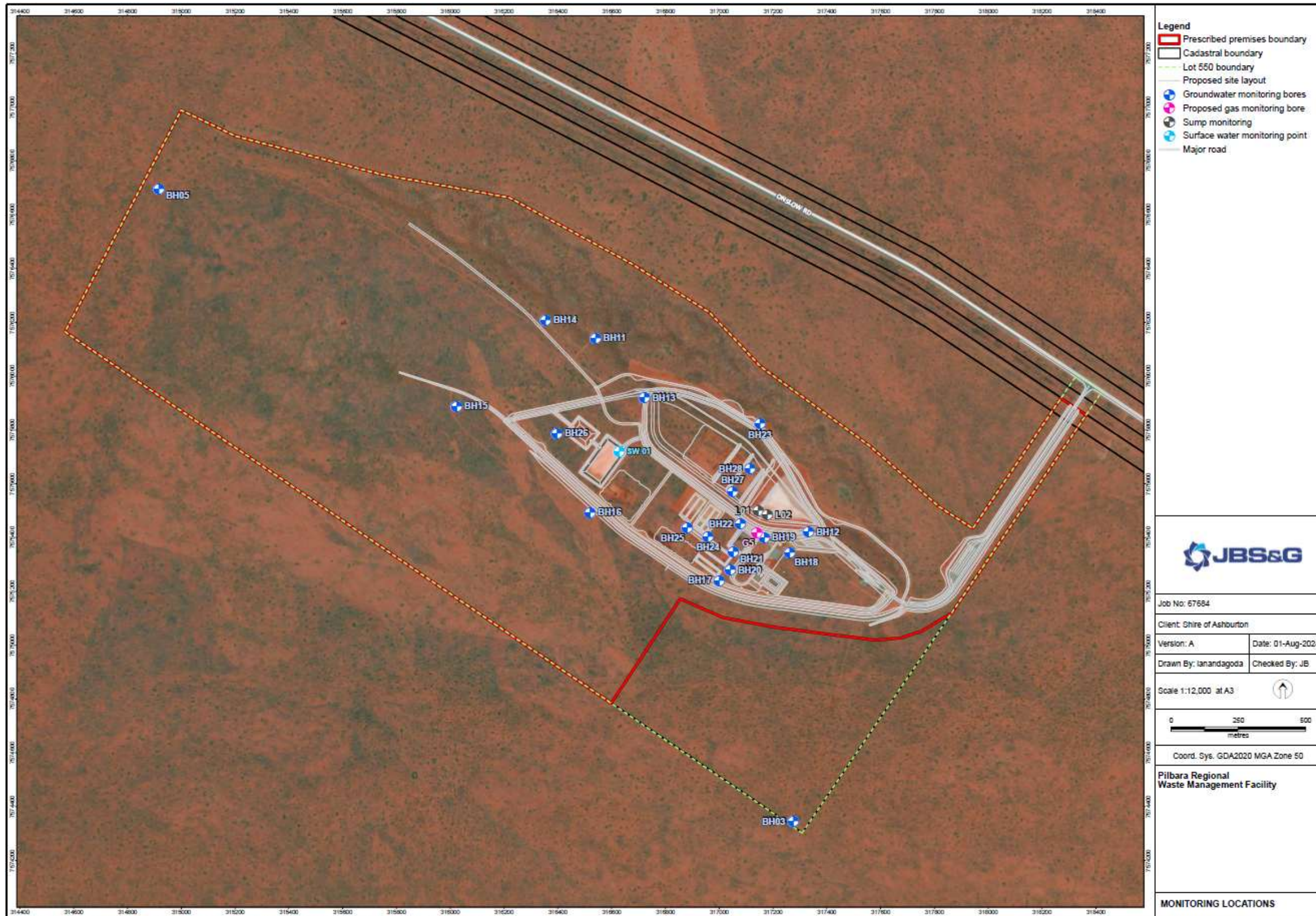
Figure 3: Monitoring bore locations.
