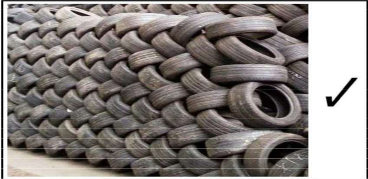
Figure 4: Laced storage of tyres.
