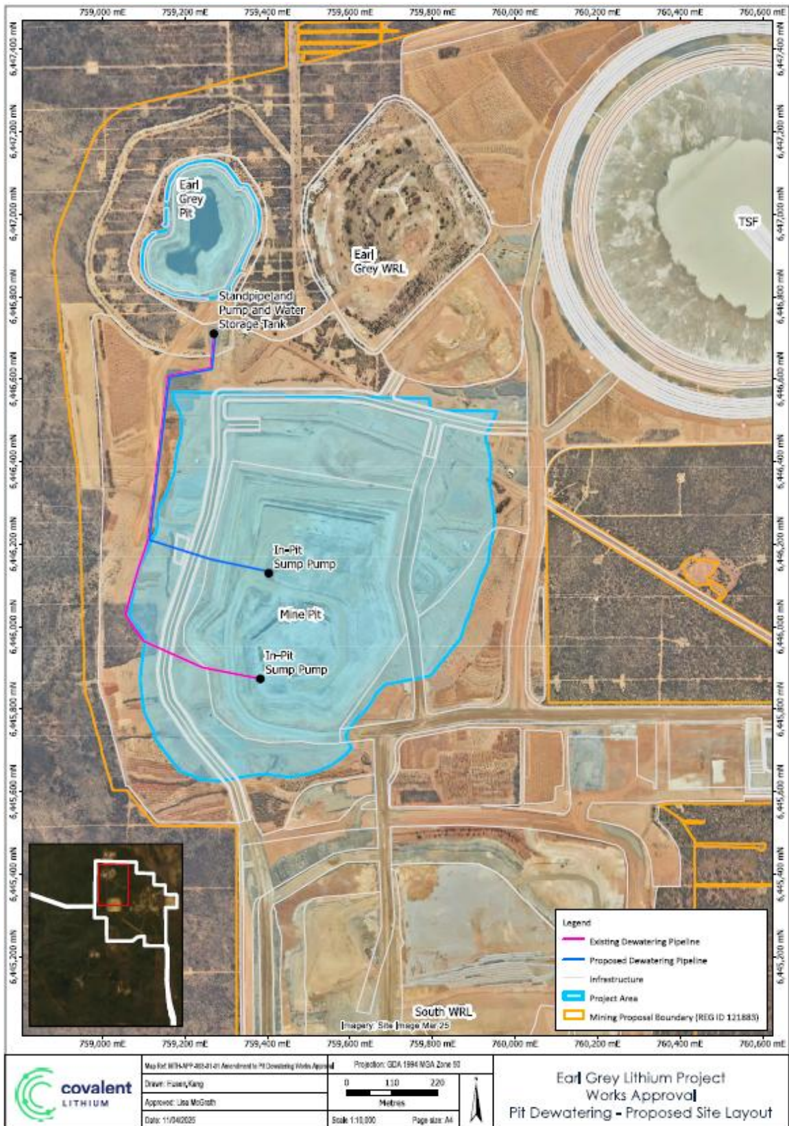
Figure 2: Layout of Dewatering Pipeline and Discharge point
