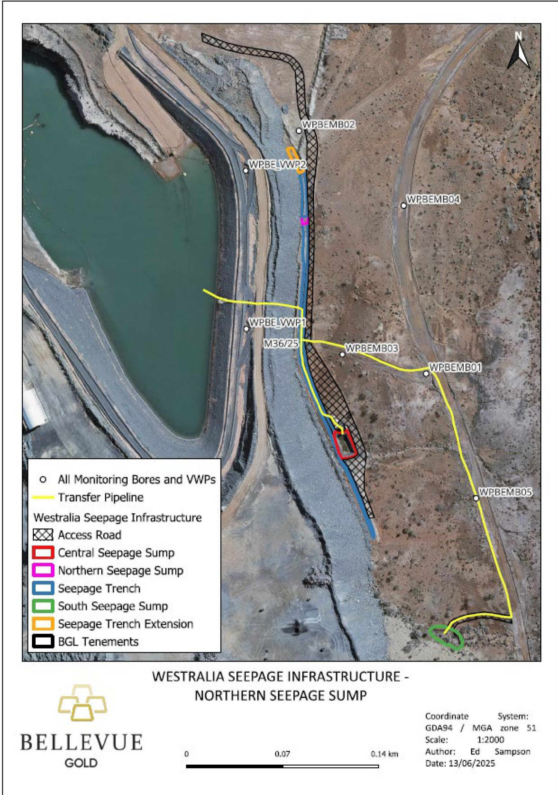
Figure 6: Westralia Pit berm expansion seepage management infrastructure
