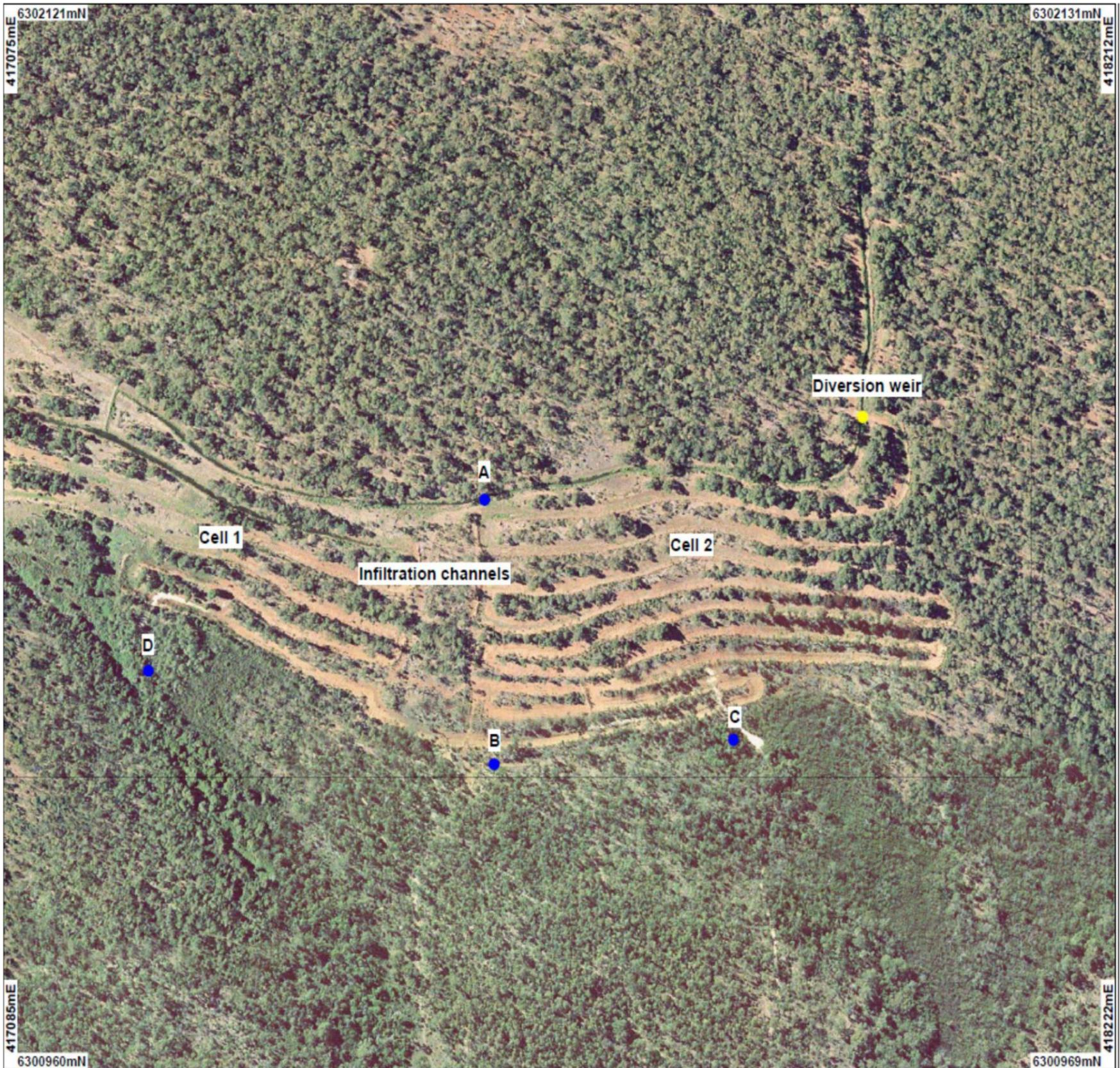
Figure 5: Location of Ambient Groundwater monitoring bores and infiltration channels
