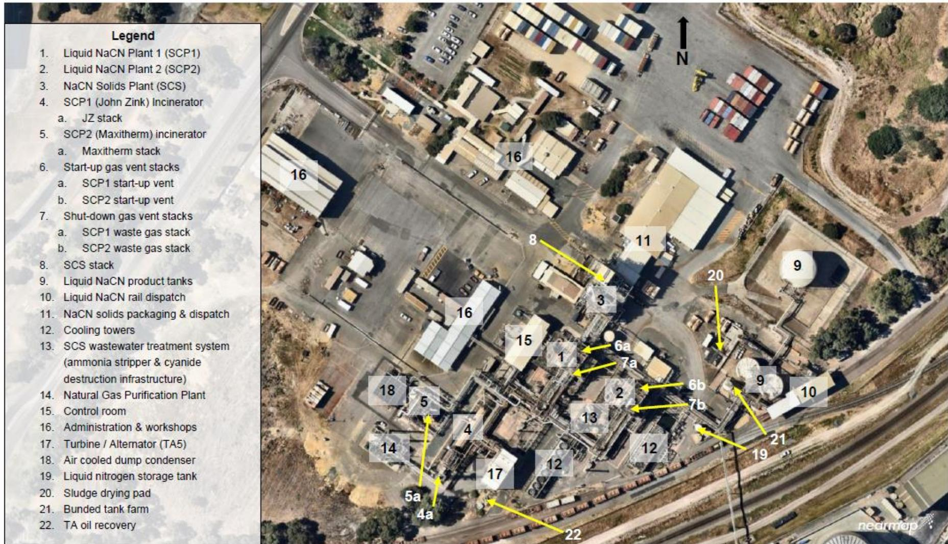
Figure 2: General layout of Sodium Cyanide Manufacturing Facility
