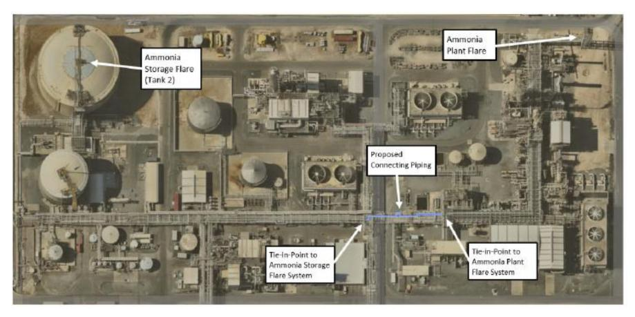
Figure 4: Proposed tie-in for Ammonia Storage and Ammonia Plant flare system
