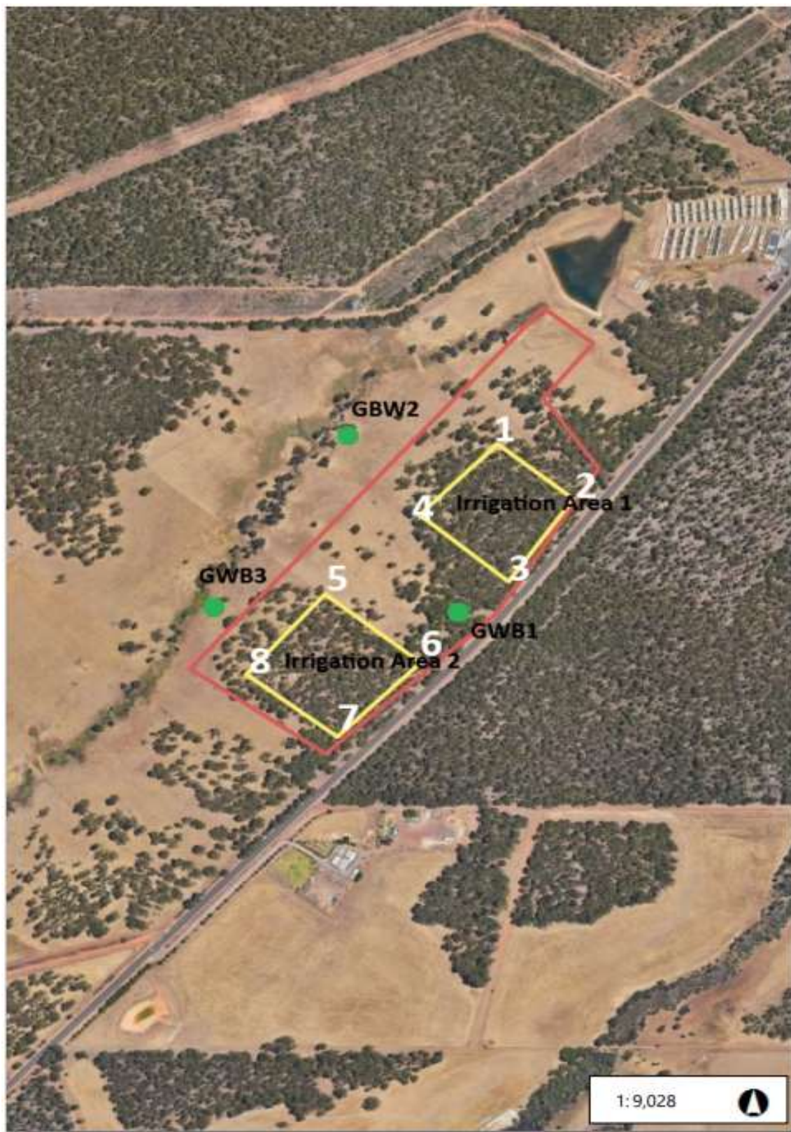
Figure 7: Groundwater monitoring bore locations (indicated in green)
