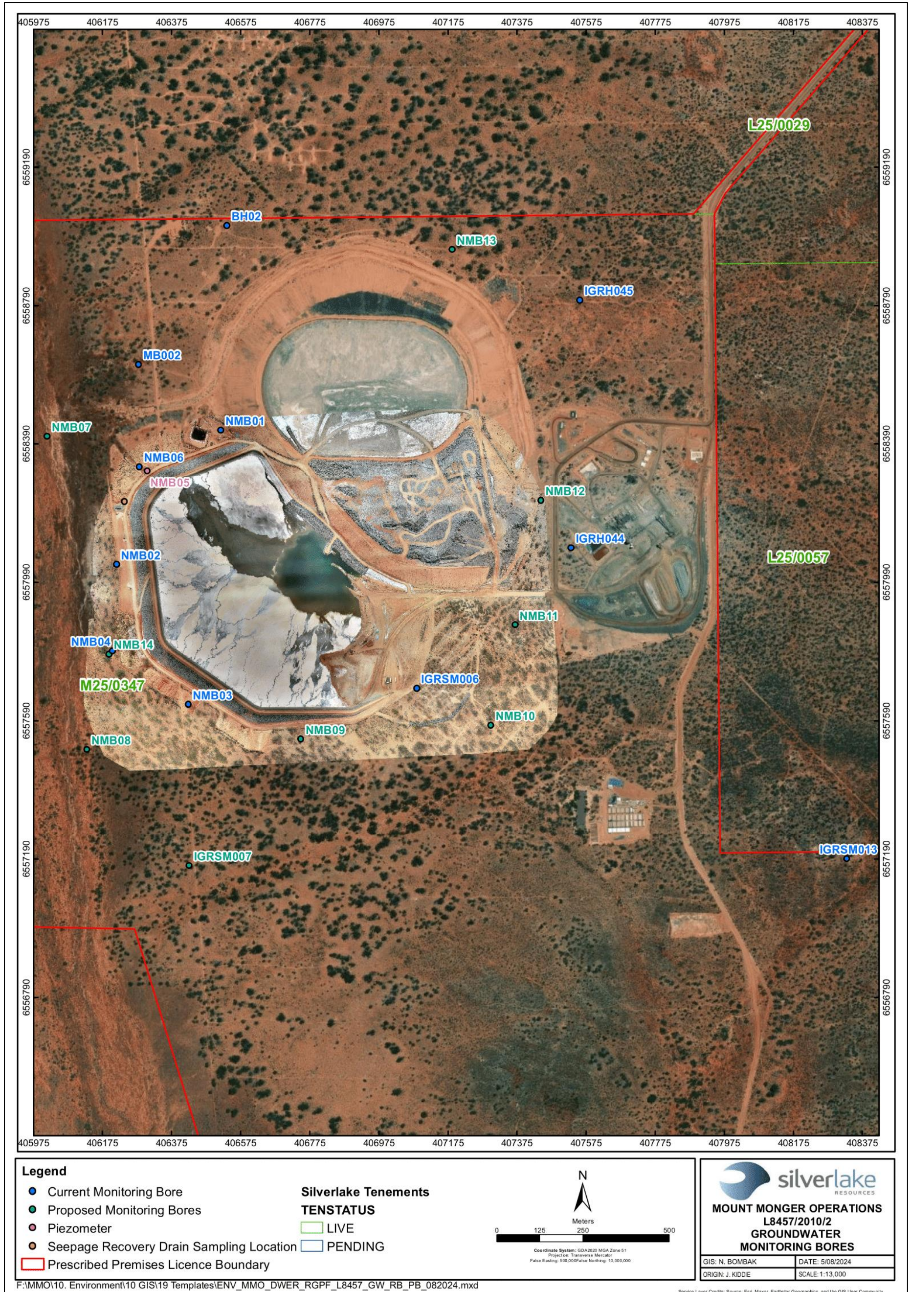
Figure 3: Proposed and existing groundwater monitoring well locations
