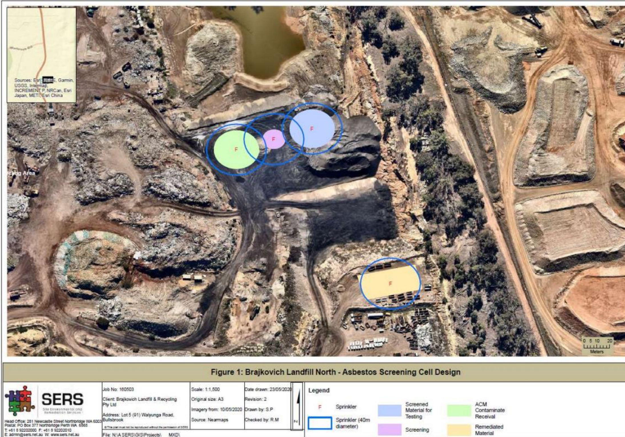
Figure 2: Map of the asbestos screening cell design
