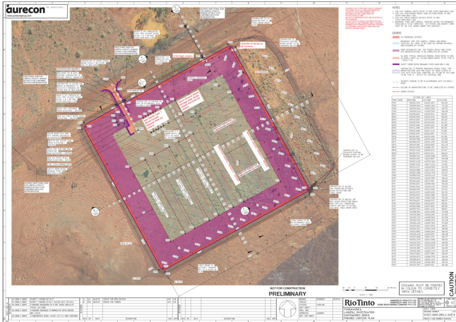
Figure 2: Landfill design (general arrangement of site infrastructure)
