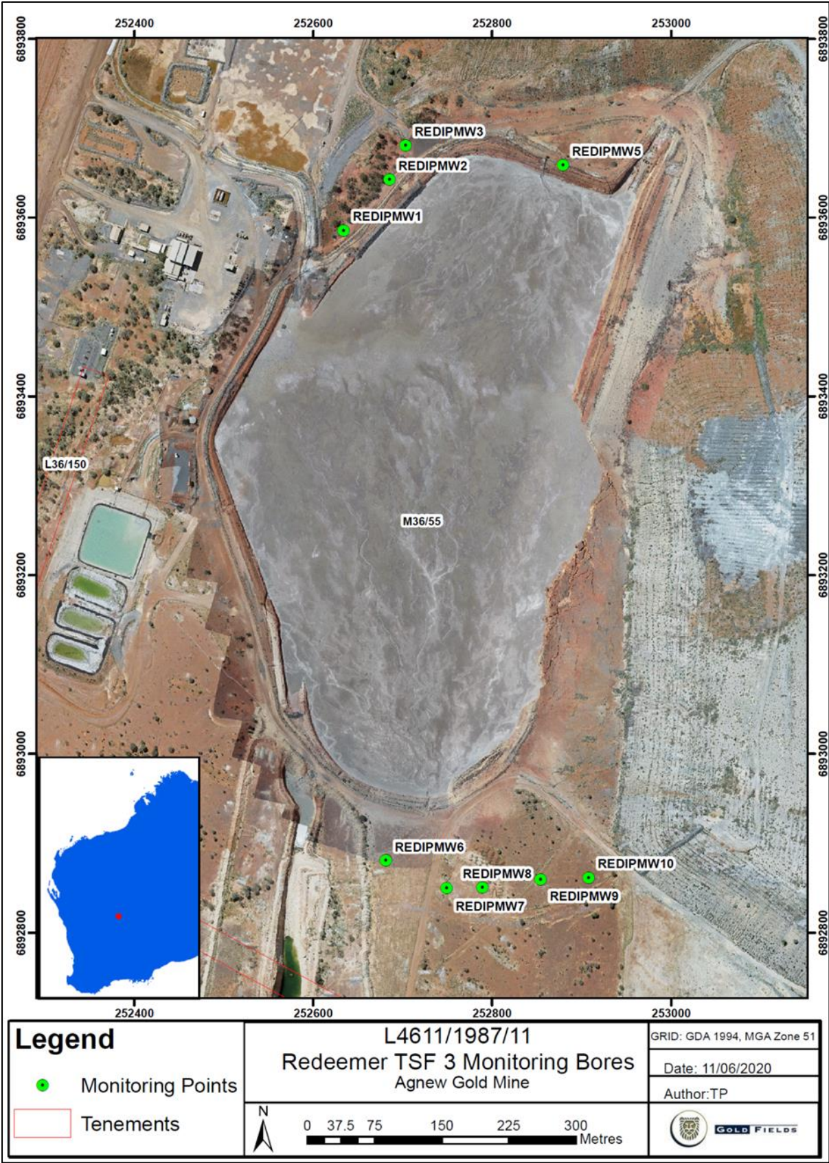
Figure 3: Redeemer TSF3 monitoring bore locations
