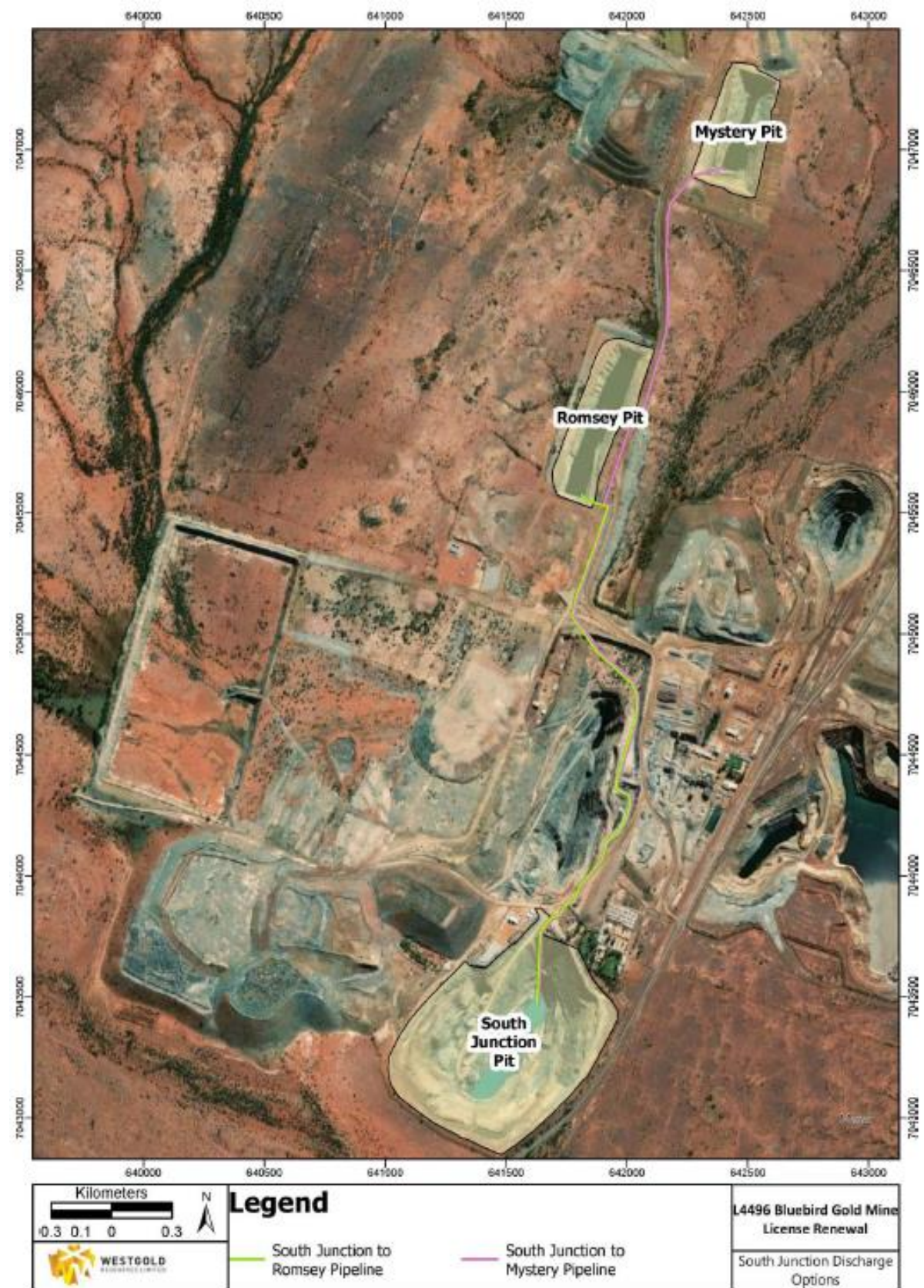
Figure 26 - Dewatering pipeline route from South Junction pit to Romsey and Mystery pits
