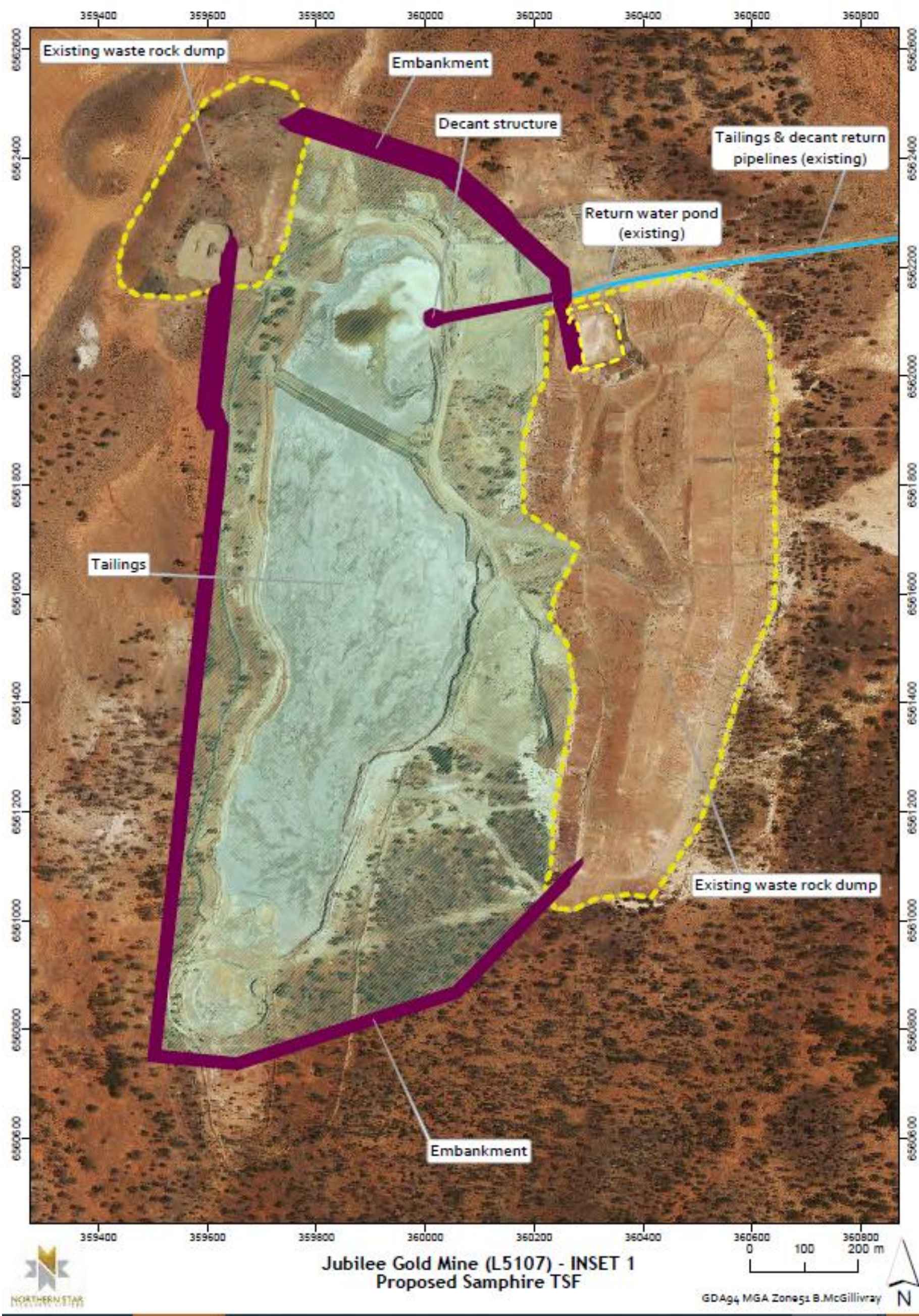
Figure 2: Saphire paddock style TSF - General Arrangement
