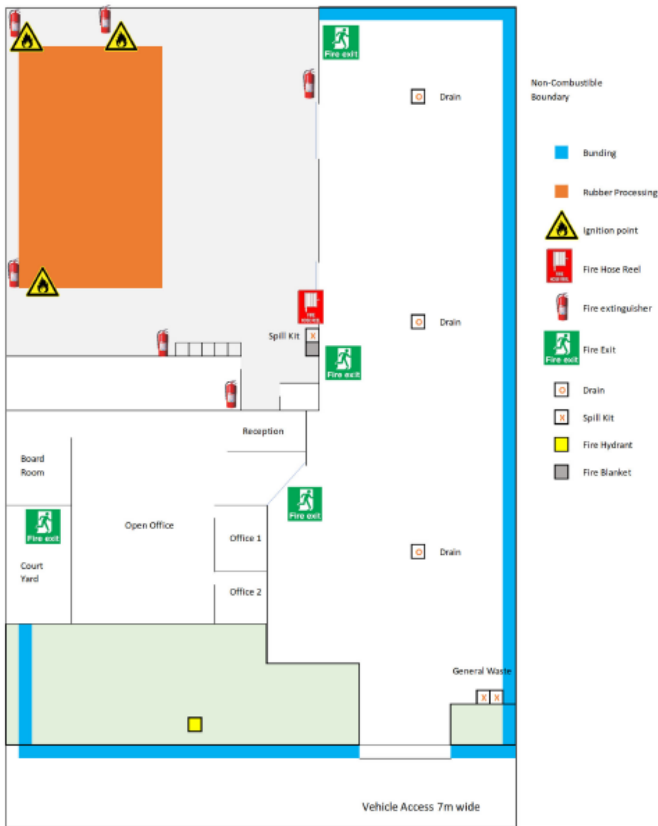
Figure 3: Surface water containment infrastructure (bundings) highlighted in blue and location of drain filter bags
