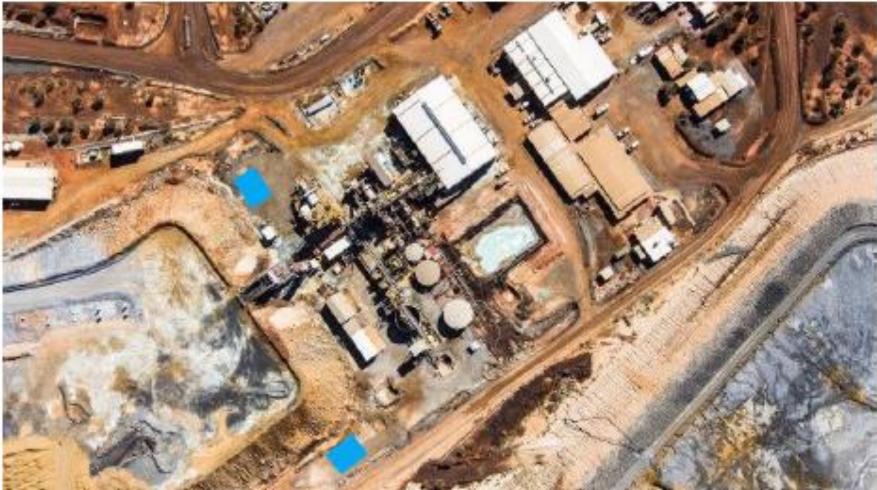
Figure 2: Close up of processing plant area and location of two new stormwater management ponds (shaded blue).
