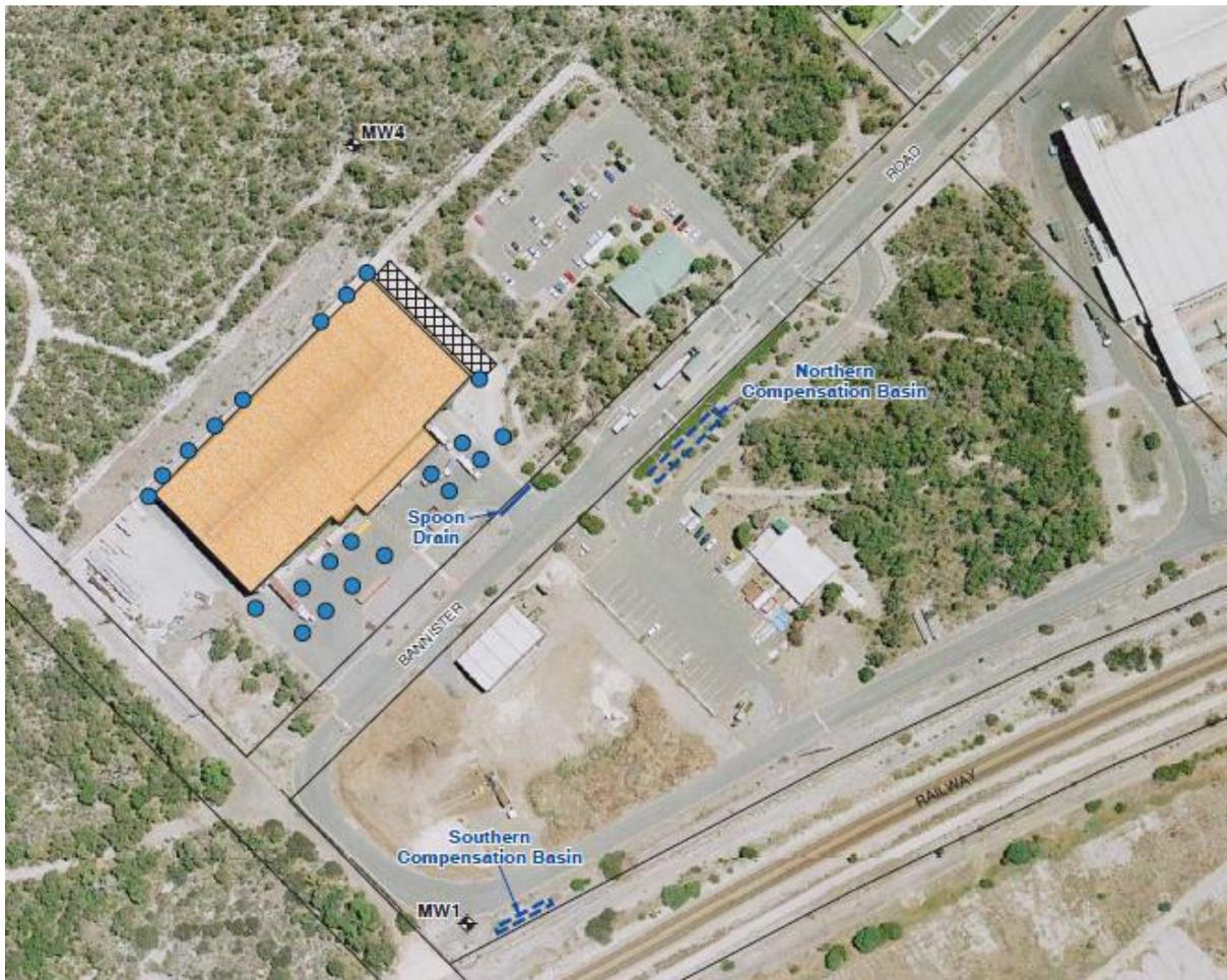
**Figure 4: Map showing stormwater and fire water soak wells (blue dots) and adjacent off site collection basins**
