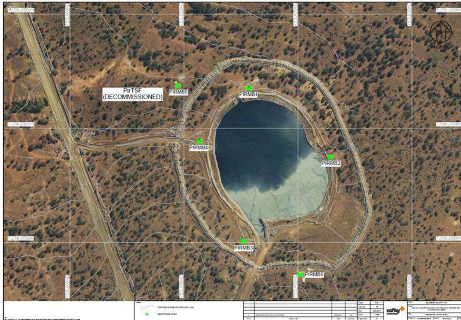
Piranha groundwater monitoring bores
