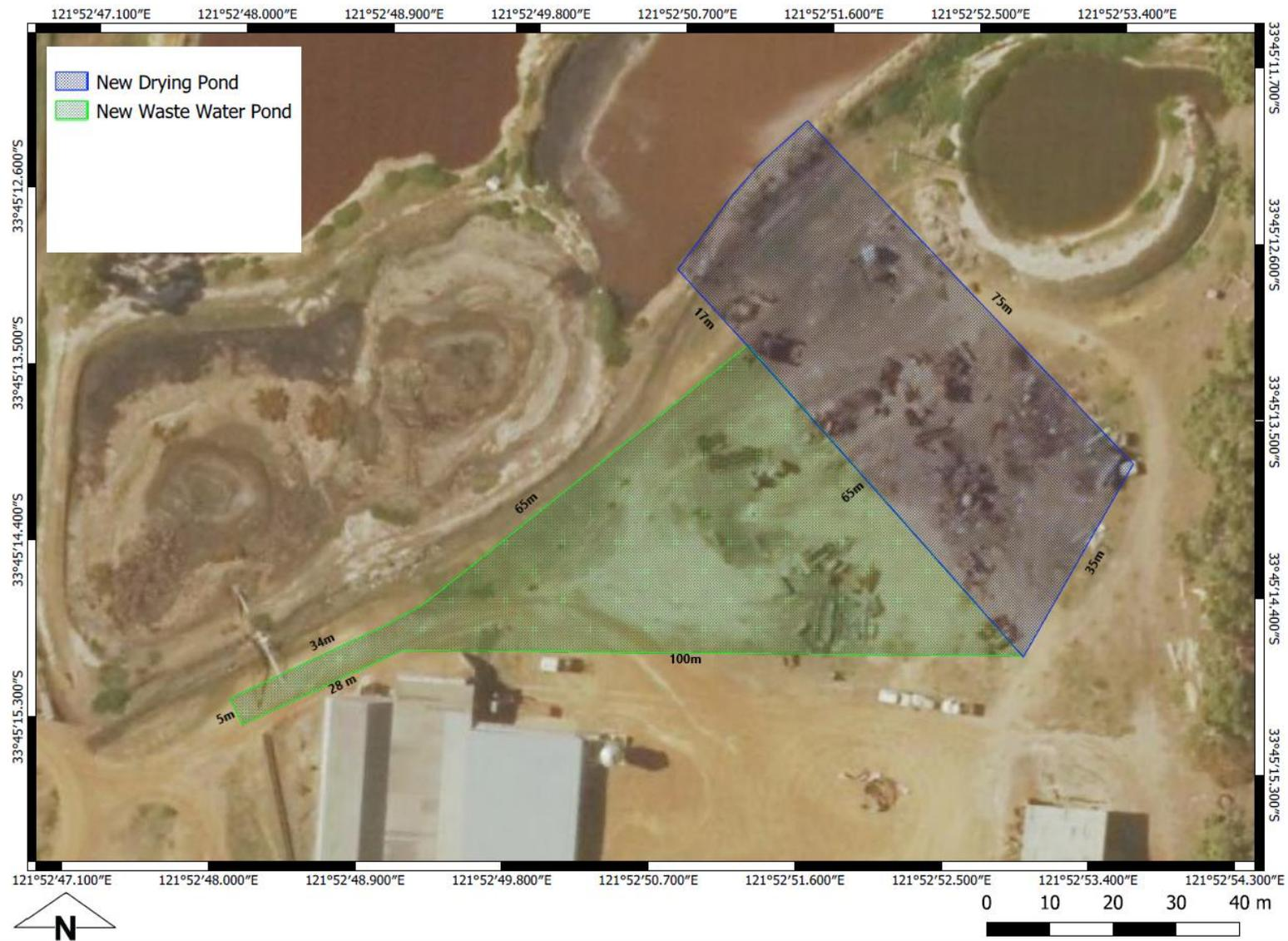
Figure 2: Layout of the proposed wastewater treatment pond and sludge drying pad
