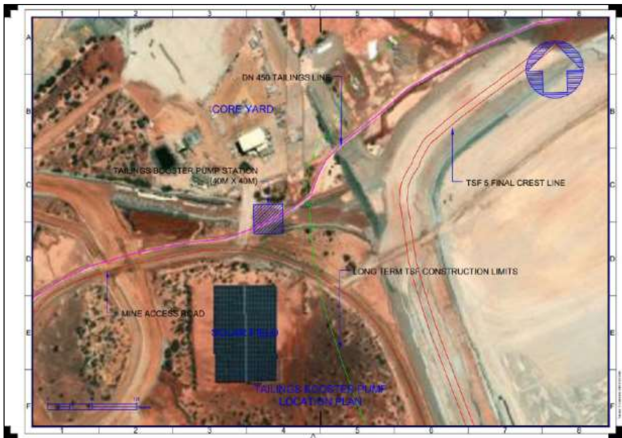
Figure 1: Proposed location of tailings booster pumping station
