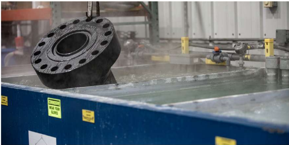
Figure 1-2: An example of a phosphating tank used to chemically coat a metal component
