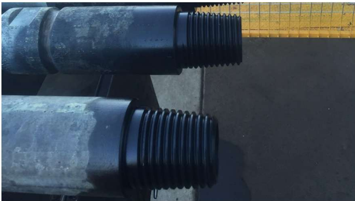
Figure 1-3: Manganese phosphate coated drill pipe connections
