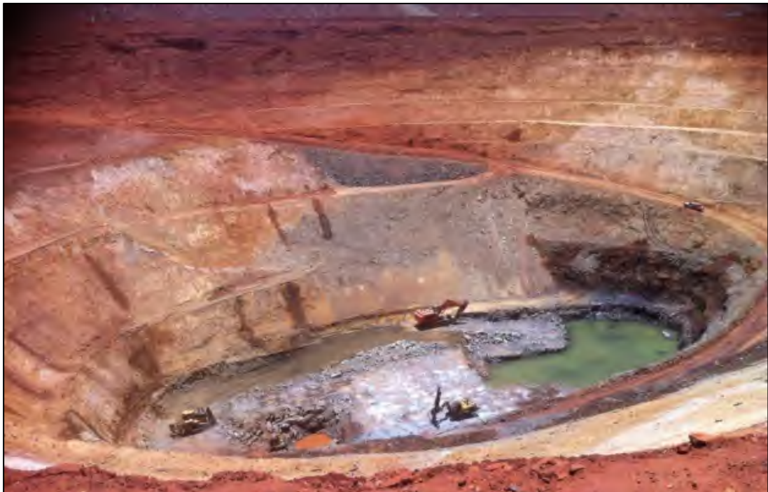
Figure 3.30: Western wall after remediation (Ramelius Image 10)
