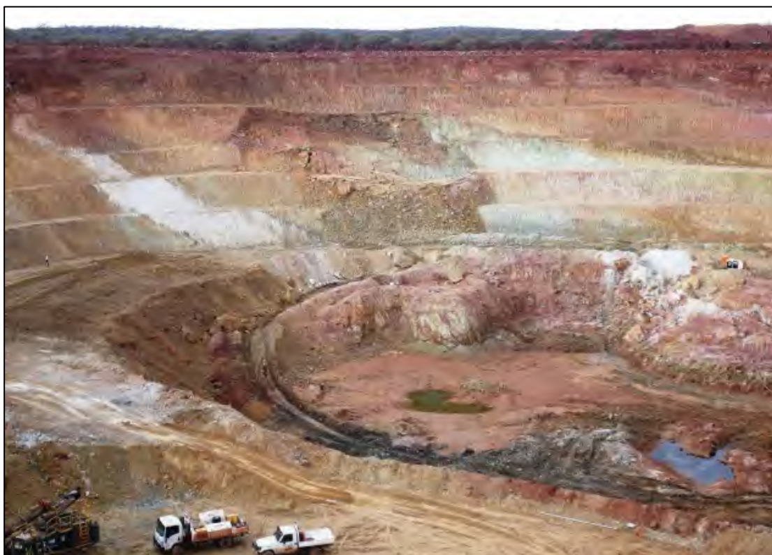
Figure 3.26: Northeastern wall failure soon after initial slump, over the next week it continued to creep and grow larger (Ramelius Image 6)
