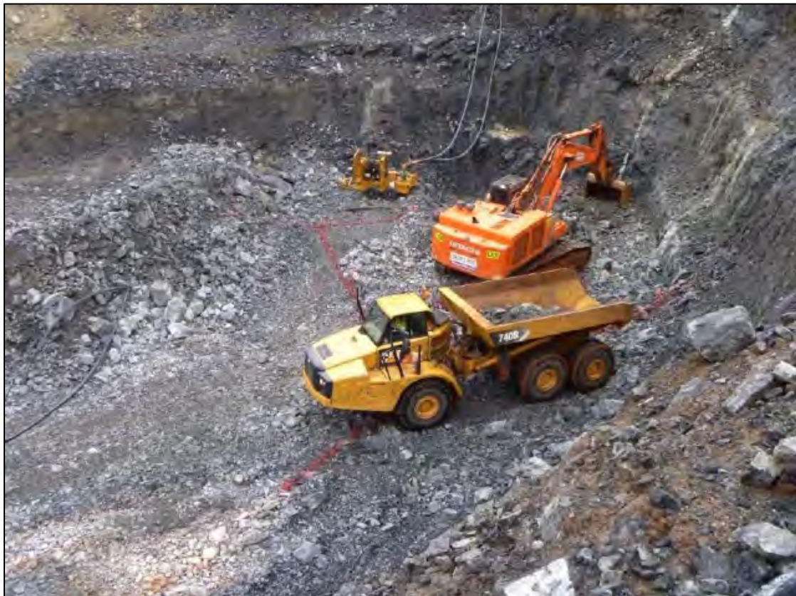
Figure 3.20: Top loading of fresh ore around 320mRL (Ramelius 2014 Image 3)
