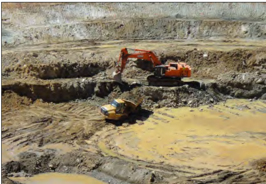
Figure 3.19: Difficult digging conditions in wet oxide material (Ramelius 2014 Image 2)
