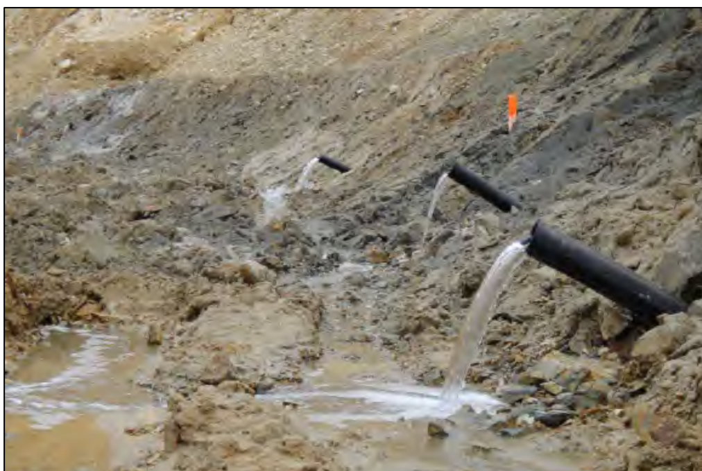
Figure 3.22: Wall holes draining water from the East on the 355 RL (Ramelius 2014 Image 4)
