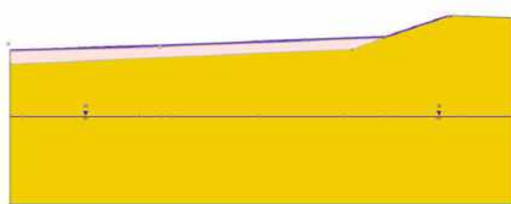
Figure 3-6: Typical North-South 1V:3H Section
