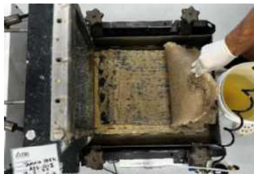
Complete delamination in 300mm x 300mm confinement zone
