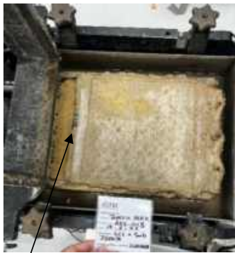
Bunching of GCL at trailing edge
