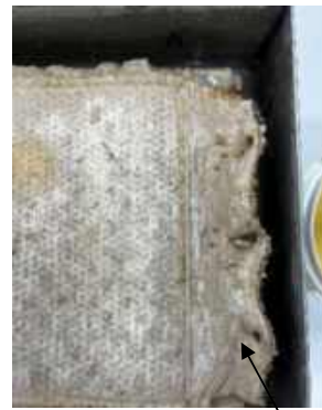
"necking" of GCL and Hole Elongation along clamped edge
