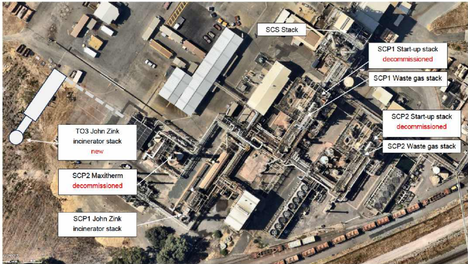
Figure164: Plot plan of site identifying discharge point at the SCMF after upgrades have been completed
