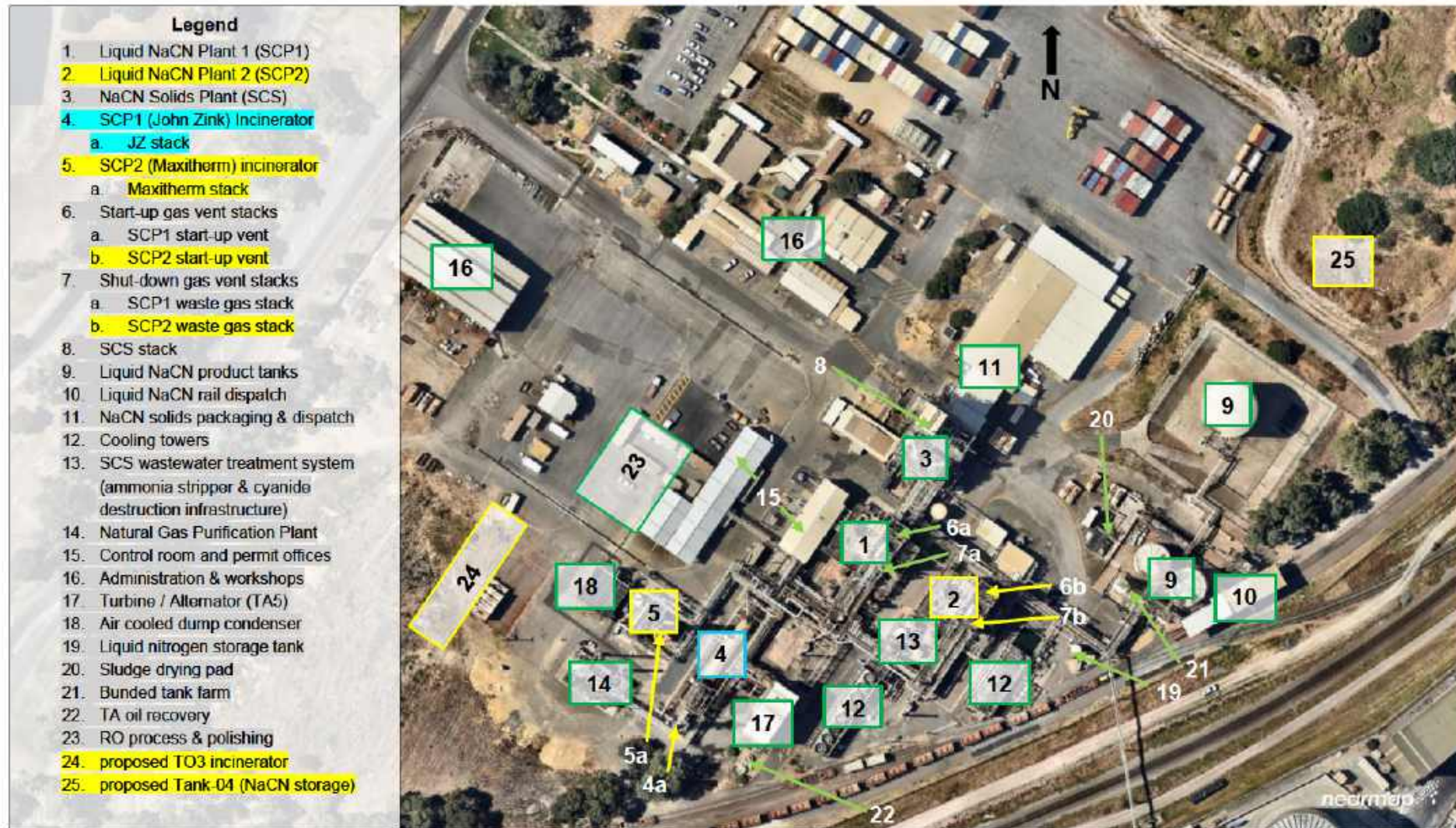
Figure 5: General layout of Sodium Cyanide Manufacturing Facility (yellow items form this application, blue items Stage 1 amendment)
