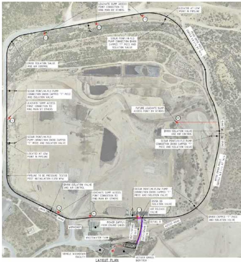
LEACHATE PIPELINE AND TANK FARM LAYOUT
