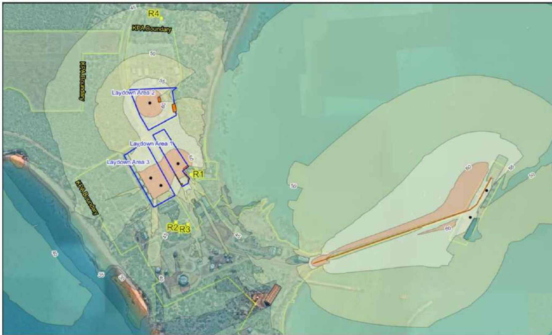
Figure K: Scenario B noise contours – KPA mineral sand loading, Barriers B
