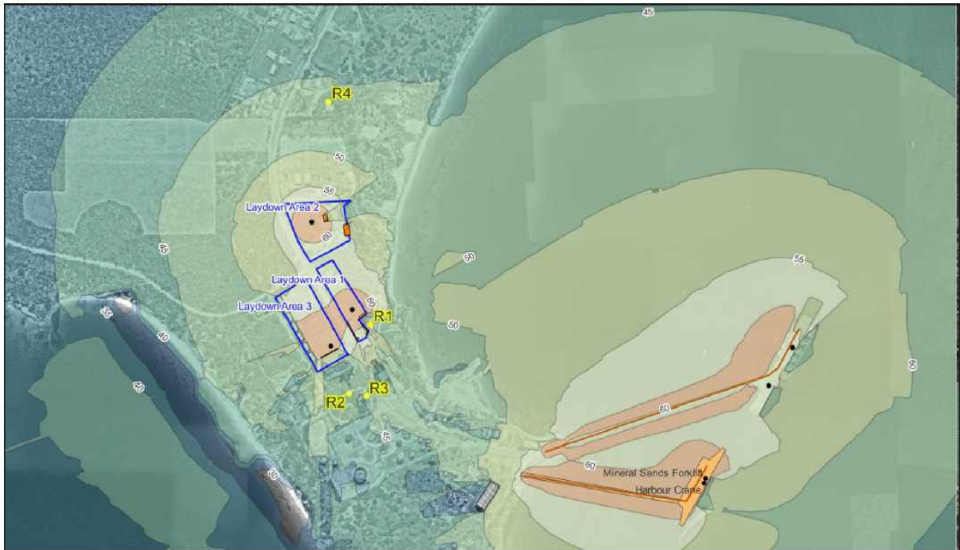
Figure I: Scenario SC2 noise contours – KMSB and KPA Mineral Sands Loading: Barriers C
