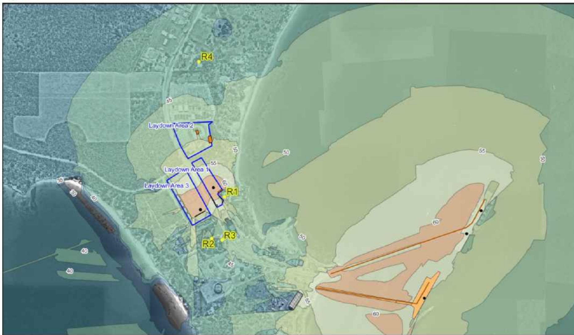
Figure M: Scenario SC4 noise contours – KPA Mineral Sands Loading / KMSB Fodder Loading: Barriers C
