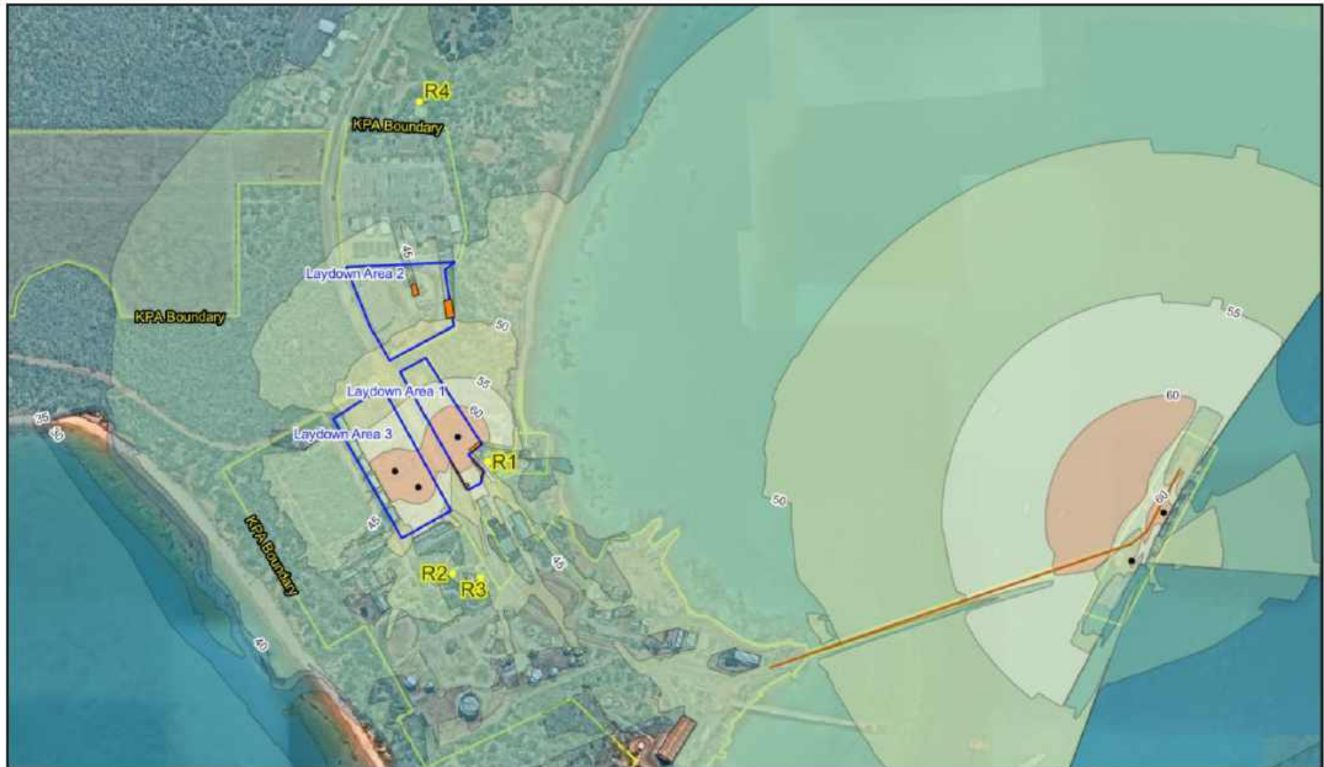
Figure I: Scenario A noise contours – fodder loading, Barriers B
