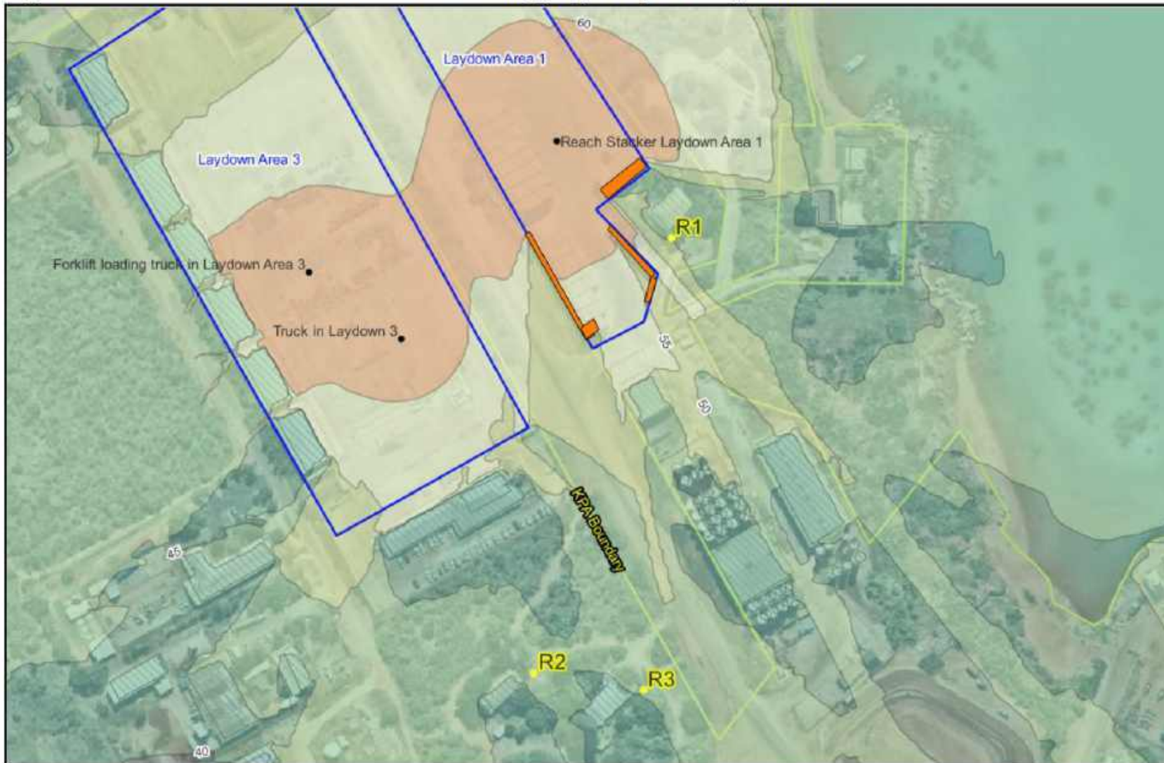
Figure J: Scenario A noise contours – fodder loading (Key Receptor Area), Barriers B
