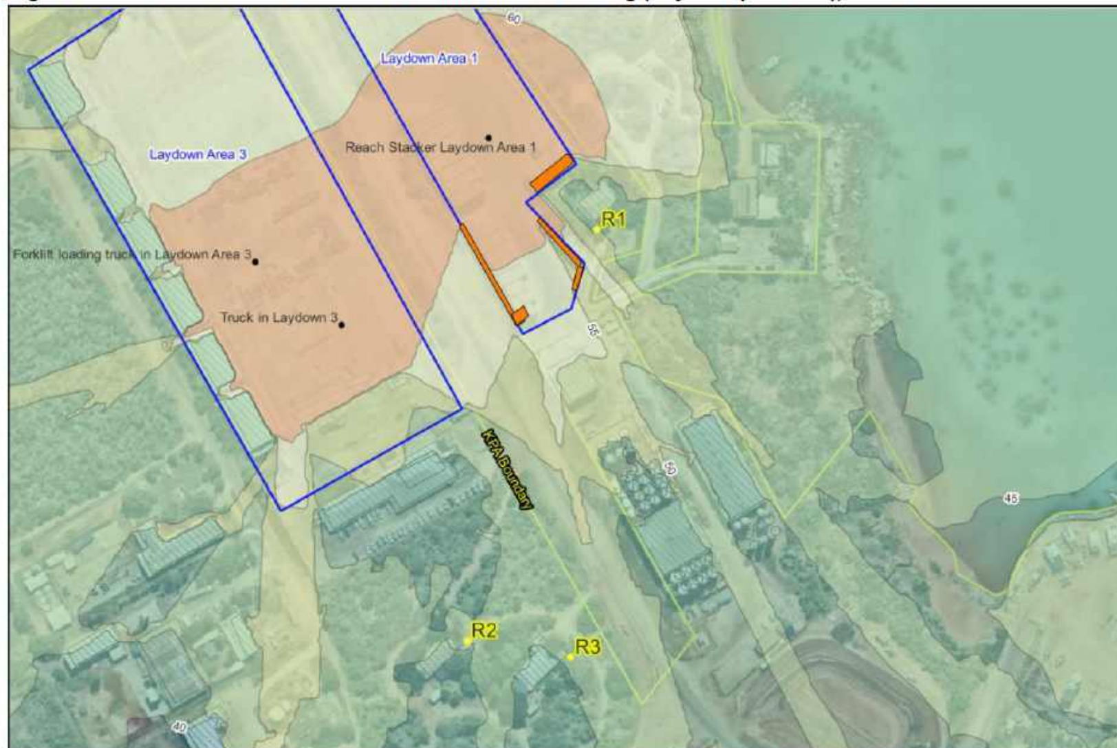
Figure L: Scenario B noise contours – KPA mineral sand loading (Key Receptor Area), Barriers B
