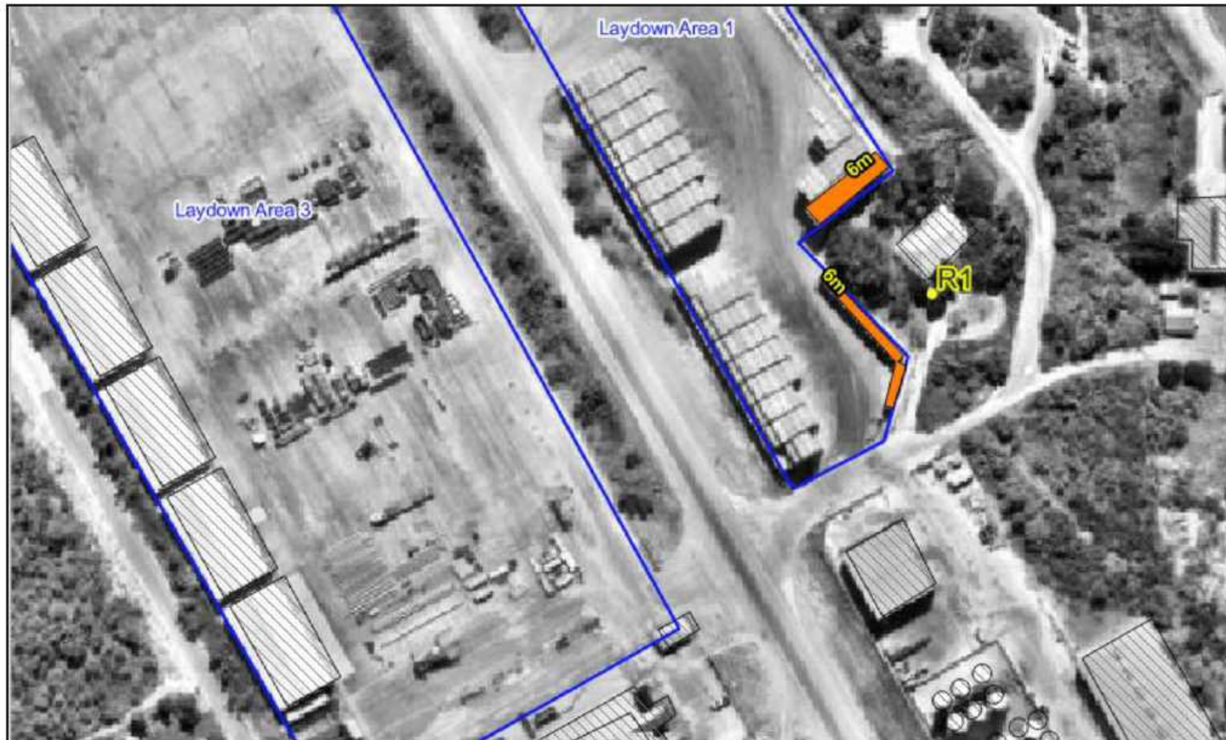
Figure E: Designated Base Barriers (3 retainers high, 6m) for Noise Mitigation Day / Evening – R1
