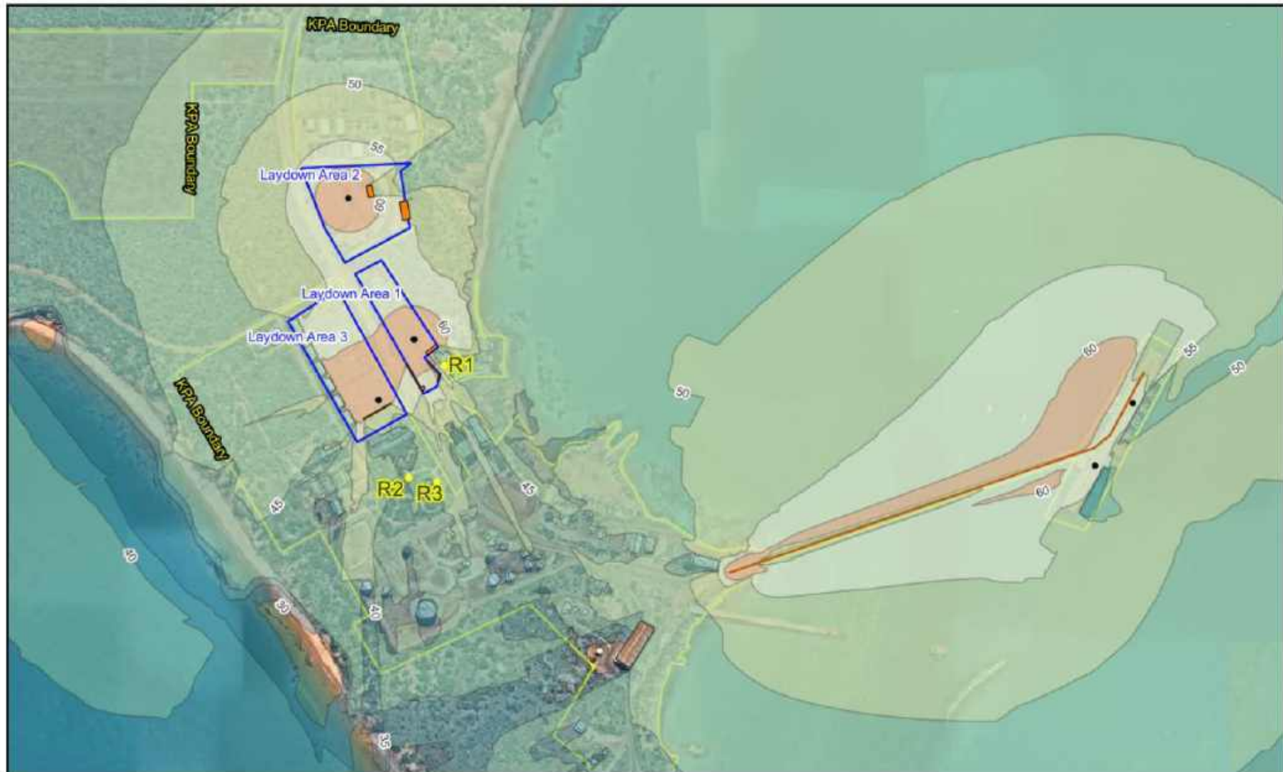
Figure M: Scenario C noise contours – mineral sand loading – All Laydown Areas, Barriers C
